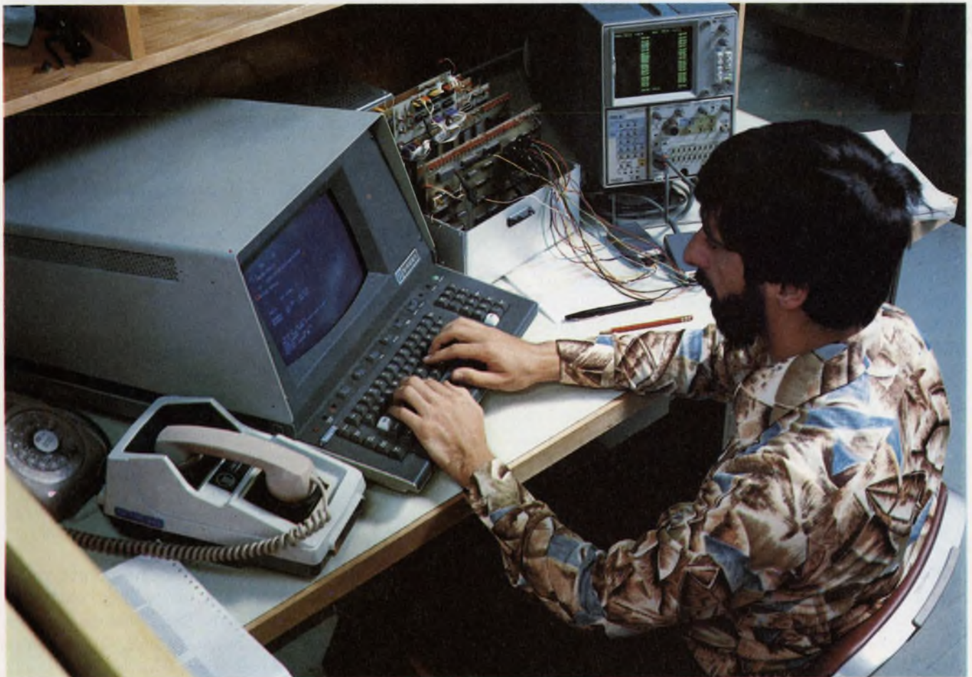
Combine logic analysis with real-time troubleshooting: Two scope plug-ins, the Tektronix 7D01 and DF1, provide
