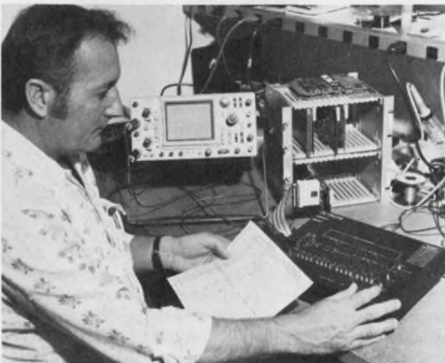
Dedicated analyzers, like the Pro-Log M822A, offer still another choice. The 822 is targeted towards the 8080, and serves as a control panel, program monitor and program-to-hardware integrator.
