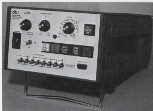
Another unit that works in real time or with digital data is Digital Laboratories' 80M. The 8-channel unit can memorize 1024 bits per channel. The static memory is said to ease output-device interfacing.
