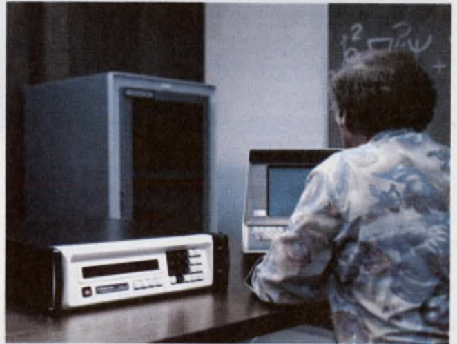
Up to 10 of these Wavetek Model 172 programmable function generators can be controlled at one time through a 488 interface with optical isolation.
