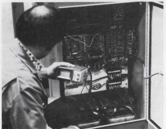
Combining both a DMM and a scope into a small, hand-held package, Tektronix' Model 213 uses the CRT to display the DMM reading.
