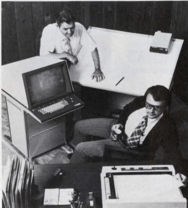
A microprocessor-based digital plotter, the Tektronix 4662, is a leader in the trend to provide plotters with the IEEE 488 general purpose interface as standard.
