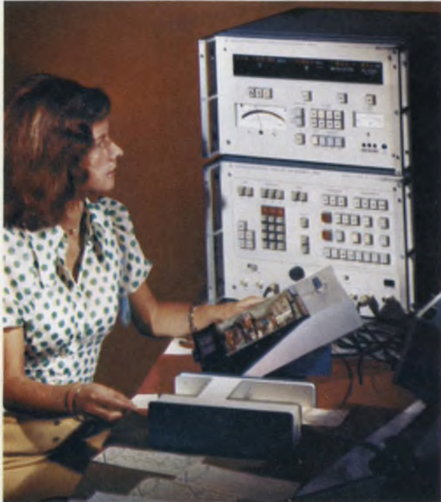
This automatic test set for transceiver measurements, by Rohde & Schwarz, is controlled through the IEEE bus by a programmable calculator. Card readers can also be used for system control.
