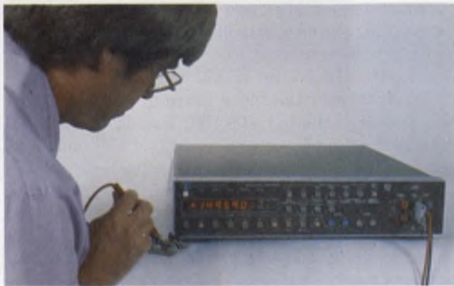
Two \mu P's in the Hewlett-Packard smart DMM control measurements, compute correction factors, handle the HP-IB interface and perform mathematics.
