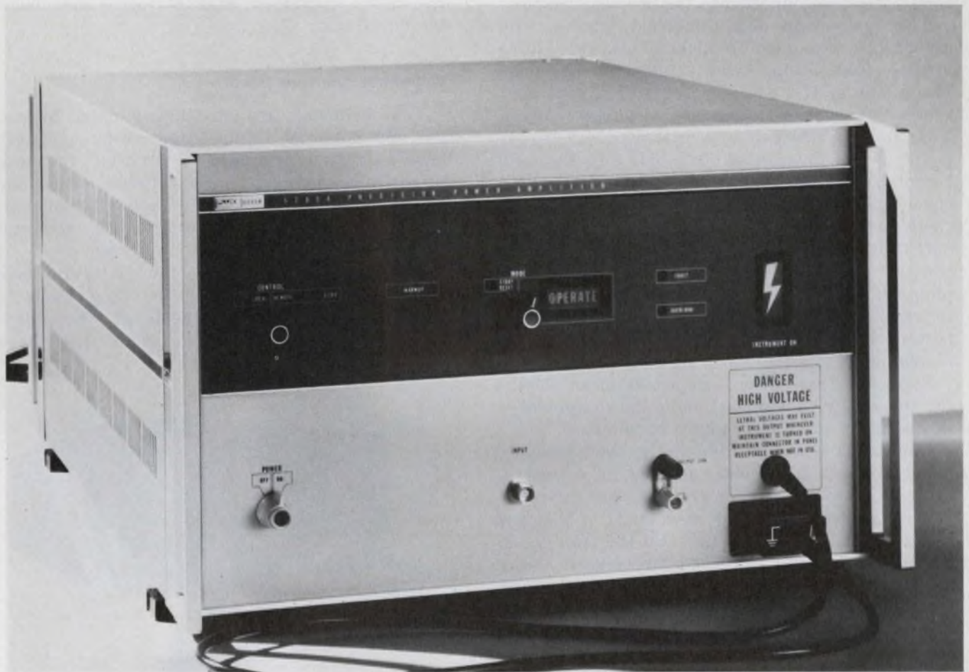
A lighted warning label that tells the user to be careful of high voltages is a new safety feature that is starting
