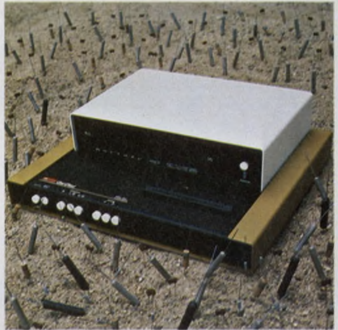
Microprocessor-directed ranging removes the guesswork in this automatic bridge, the GenRad 1657. Maximum resolution is always achieved on the readout.
