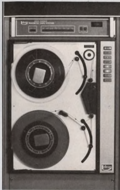
The 4600 mag tape system uses an 8080 \mu P for tape control.
