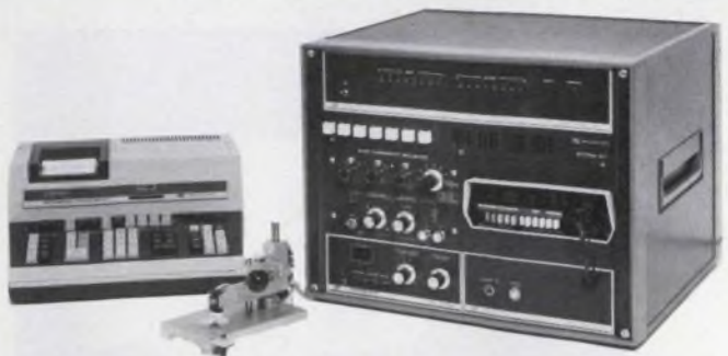
A calculator-controlled automatic test system for four-point probe applications, the Keithley System 53 contains a current source, DMM, 10-channel scanner and interface units.
