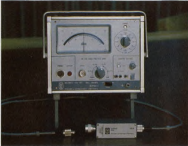
Accurate rms measurements at zero dBm and zero dB levels are provided by W & G's EPM-1 milliwatt test set. Probe circuitry prevents thermocouple burn-out.
