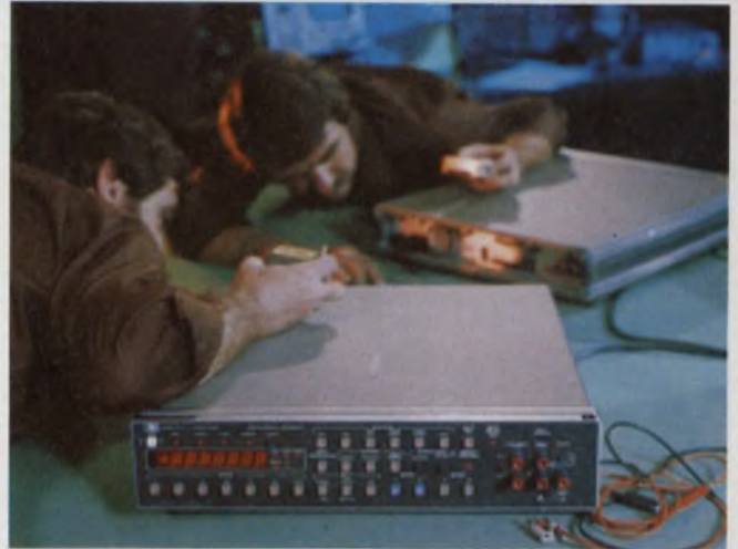
Removable reference assembly simplifies calibration of dc functions and ohms in Hewlett-Packard's 3455A, a guarded integrating 5-1/2 or 6-1/2-digit multimeter.
