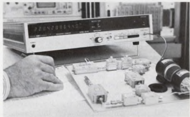
Fully automatic frequency measurements from 0.02 to 24 GHz can be made with this Systron-Donner 6054B Microwave Counter. The IEEE interface is optional.
