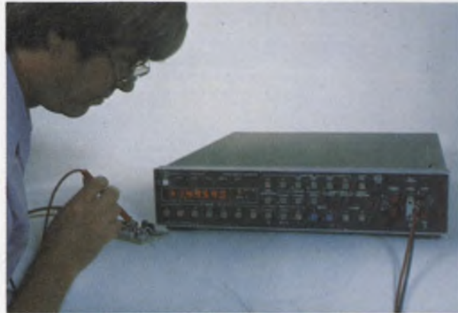
The status of the HP-IB bus as well as the range and the function to which the meter is set are provided automatically by this Hewlett-Packard 3455A DVM.
