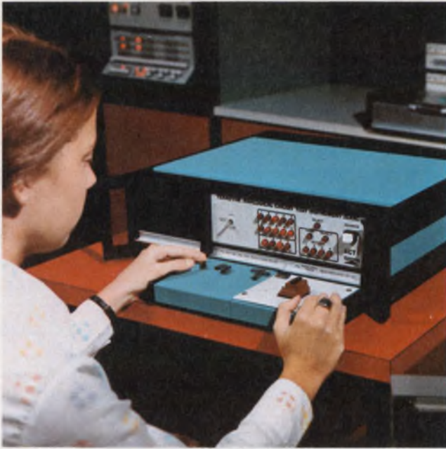
You can check 5000 different ICs on Teradyne's J133 digital tester. The unit never needs calibration, and can interface with an automatic handler.
