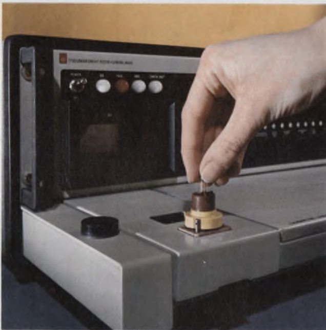
Testing of linear circuits usually requires measurement of a fair number of circuit parameters. GenRad's 1730 sets test limits with a programmable memory panel.
