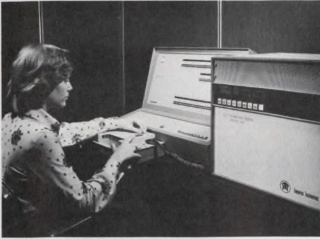
Two testers team up to provide 10-MHz functional check-out and dc-parametric memory tests (Siemens).
