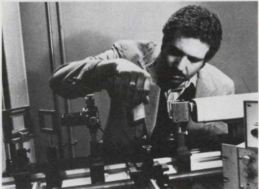
A He-Ne radar version of the three-frequency heterodyne system is adjusted by Dr. Malvin Teich.
