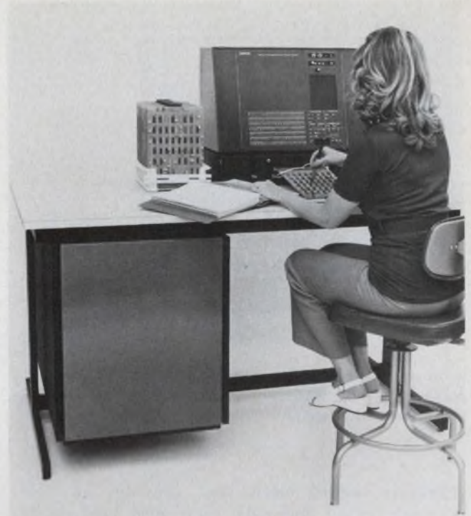
Microprocessor-based testers, such as this one from Mirco Systems, give computer-like performance in a compact—or even portable—package.
