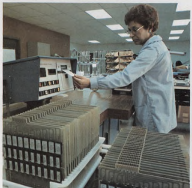
Paper-tape diagnostics identify defects on a printed-wiring assembly. The equipment is the Faultfinder's 101A, an in-circuit test system that probes solder nodes.
