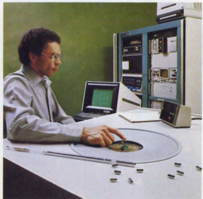
Graphic displays of test results are one benefit of computer-controlled test equipment. Evaluation of LSI circuits is shown here on the Tektronix S-3260.
