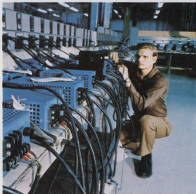
More than any other type, switching-regulated supplies need burn in and life testing to weed out infantile failures and to check new designs (courtesy of Sorensen).
