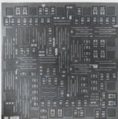
We start with a standard chip carrying unconnected components.
