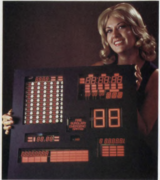
A mixture of different message formats such as alphanumeric and fixed messages can be combined into one unit using the National Electronics Plasmac display.
