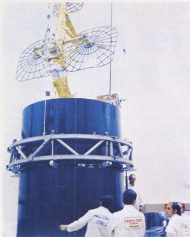
The Hughes Intelsat IV-A satellite contains 20 transponders, permitting 20 channels, each 36 MHz wide, to operate through twin 53-in. dish antennas. It uses a 4-to-6-GHz downlink and 6-GHz uplink.
