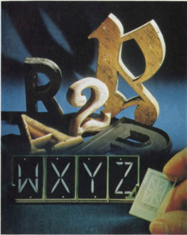
Alphanumeric characters can be displayed by 16-segment LCDs. These one-inch-high units from Hamlin can be read at 30 ft.
