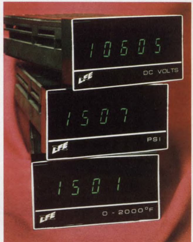
Fluorescent displays produce a pleasing green glow when lighted. They require low power and low voltage, but are susceptible to shock because of their glass package.
