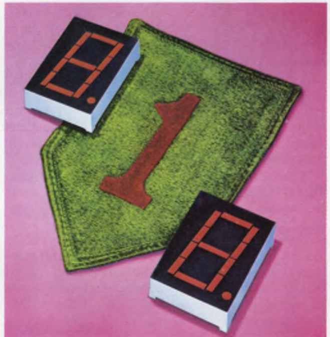
One of the first 1-in. LED displays to be announced is this one from IEE. It uses two LED chips per segment and, therefore consumes twice as much power as the small half-inch displays.
