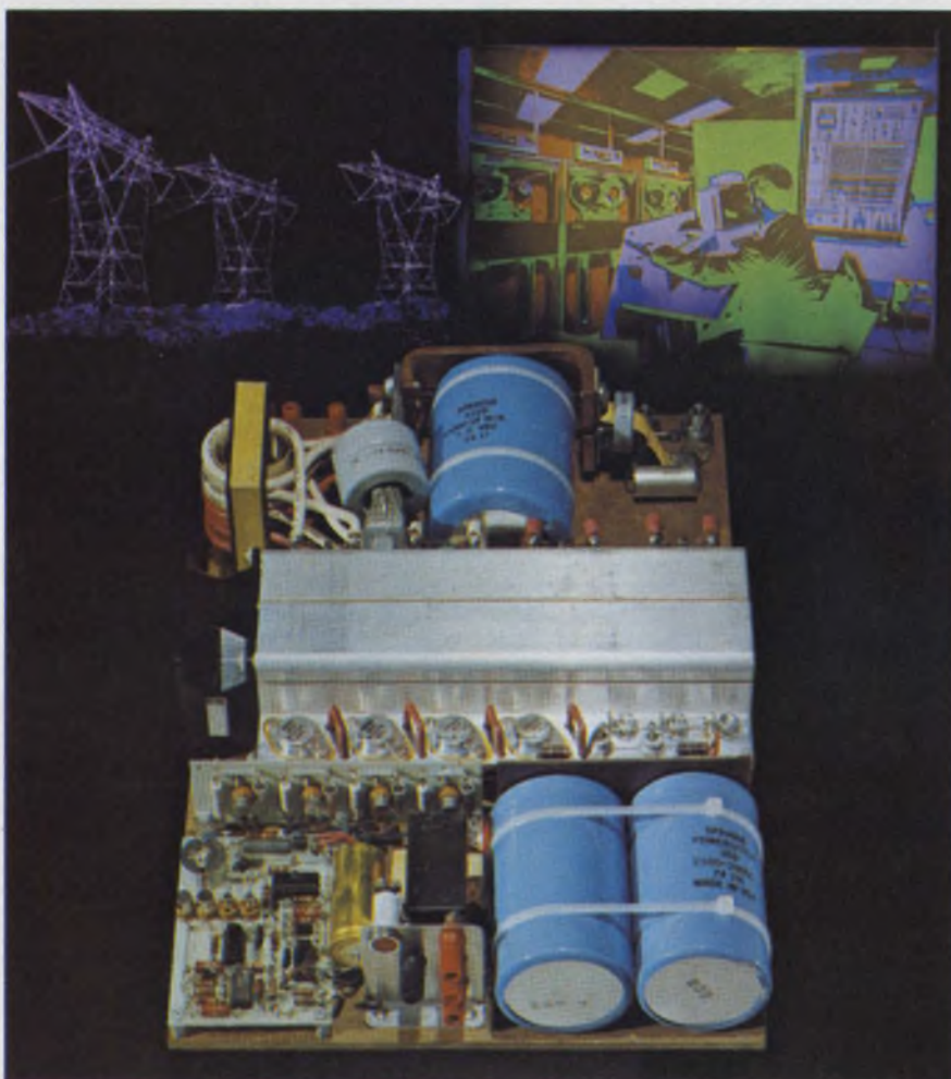
Fast-switching transistors, power Darlington transistors and Schottky diodes are key components in high-efficiency power supplies, like this 1000-W off-line unit designed by TRW Power Semiconductors. Efficiency is better than 80%.
