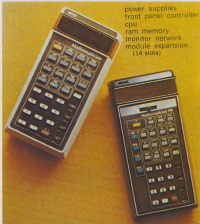
A steady reduction in the cost of scientific calculators, like these Novus machines, is being achieved through the use of fewer chips with more circuits on each chip.
