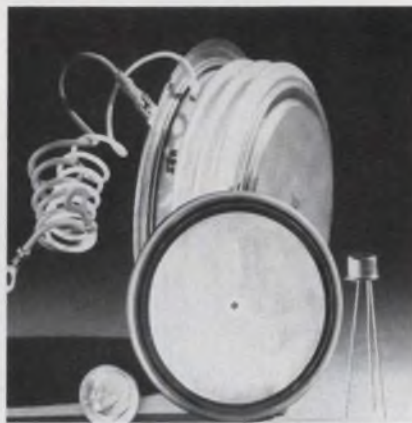
Very-large-diameter wafers , like these made by International Rectifier, carry thousands of amps.
