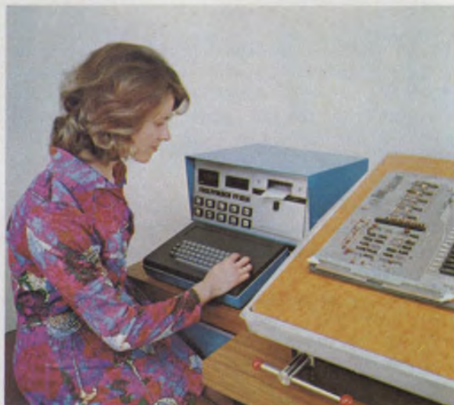
A dual magnetic tape cassette with an autosearch feature in this Faultfinder FF101A test system simplifies the programming, editing and test program debugging.
