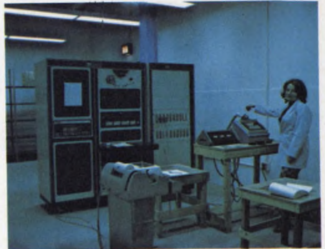
Testing the conductor patterns of bare PC boards on this Circuit-Wise computer-controlled setup has revealed a surprising number of defects not detected visually.
