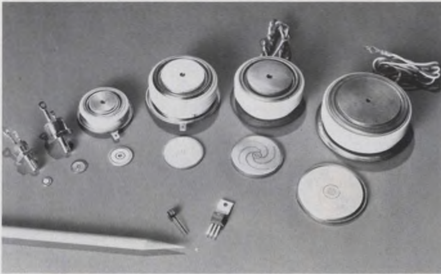
Wafer sizes for power SCRs have increased from the small, stud-mounted units made by GE in the late 1950s to the large 1 and 2-in. diameter devices available today that handle megawatts.
