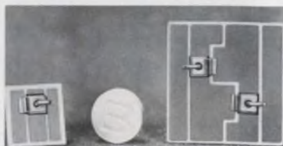
Uncased power semiconductors mounted on ceramic substrates can cut costs 40%, claims Unitrode.
