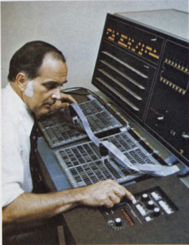
Four million 128-bit words can be generated by this Fluke-Tendar 2000A logic tester. Here, software is replaced by combination of pseudo-random codes.
