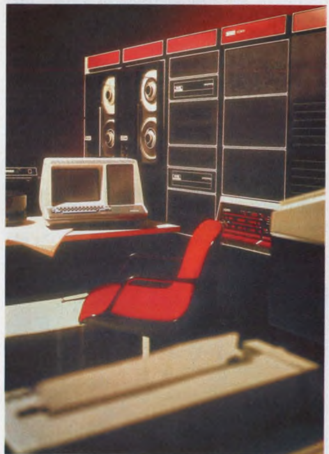
Digital Equipment Corporation's new midcomputer, the PDP 11/70, employs a special memory architecture in which a 2 k byte bipolar cache memory acts as a buffer between main memory and the unit's general purpose registers. 32-bit internal data paths carry data to and from the cache memory, permitting data transfers between memory and registers to approach the 300-ns execution time of the central processor.
