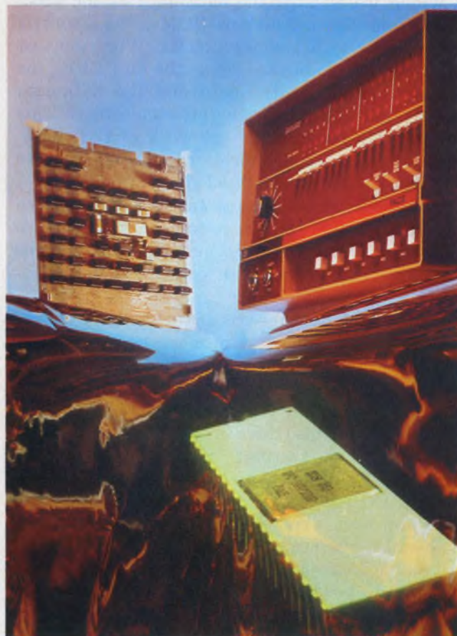
The first 16-bit microprocessor on a single chip is the Pace from National Semiconductor. It has a 45-instruction set that cannot be modified. Instruction cycle time is typically 10 \mu s . Shown also is the Pace microcomputer card prototyping systems.
