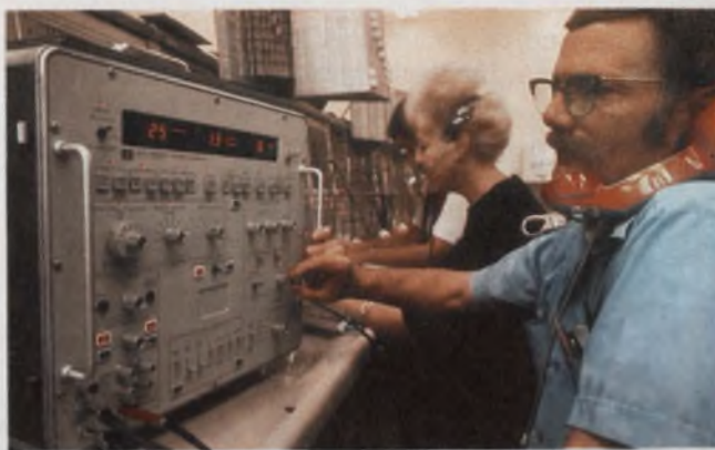
The use of telephone voice channels for digital data transmission requires special line quality measurements. This Hewlett-Packard 4940A Transmission Impairment Measuring Set separates and simultaneously measures six types of transient line disturbances.
