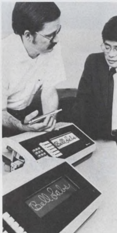
Flat-screen plasma panel transmits photographs, drawings and writing to remote panel by telephone wire.
