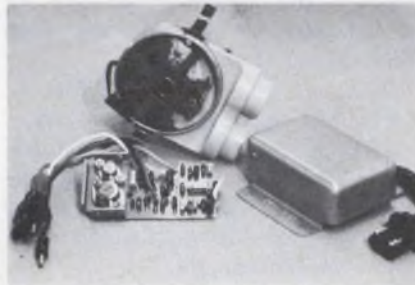
Electronic ignition hardware consists of distributor with trigger wheel, printed-circuit board with IC, sensor coil (mounted on distributor housing) and enclosure.
