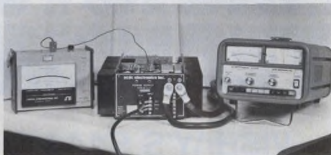
Core temperature is easy to measure with a thermocouple attached to the capacitor's positive terminal.
