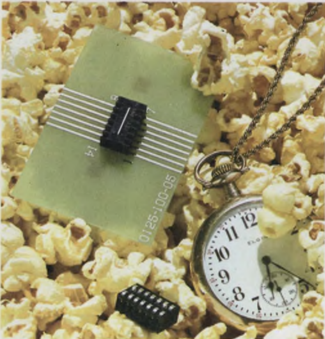
No soldering and little drilling are characteristics that describe ITT Cannon's Popit socket. C-shaped contacts apply pressure to the IC and connect to PC traces when the socket is forced into the board. Two metal staples hold the socket.
