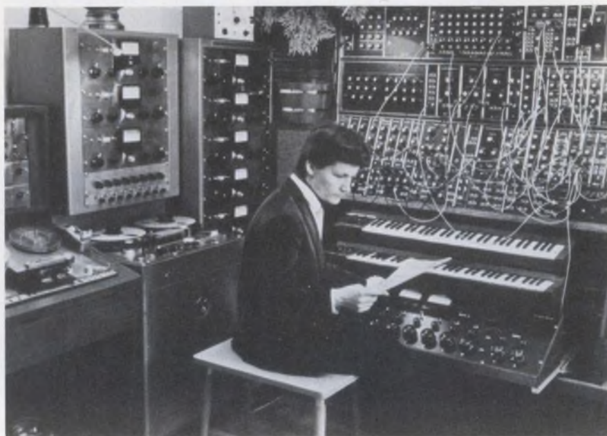
With this installation, Walter Carlos, an ex-studio recording engineer, produced the "Switched-On Bach" record in 1968—the first commercially successful synthesized recording. To the left is an eight-track recorder and to the right is his custom Moog synthesizer and mixing panel.
