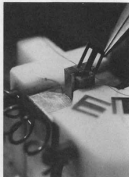
tion. Here skilled operators, using microscopes of 10 to 30 power magnification, are stacking tiny laminations in the bobbin of a Bourns 1/4-in.-cube transformer.
