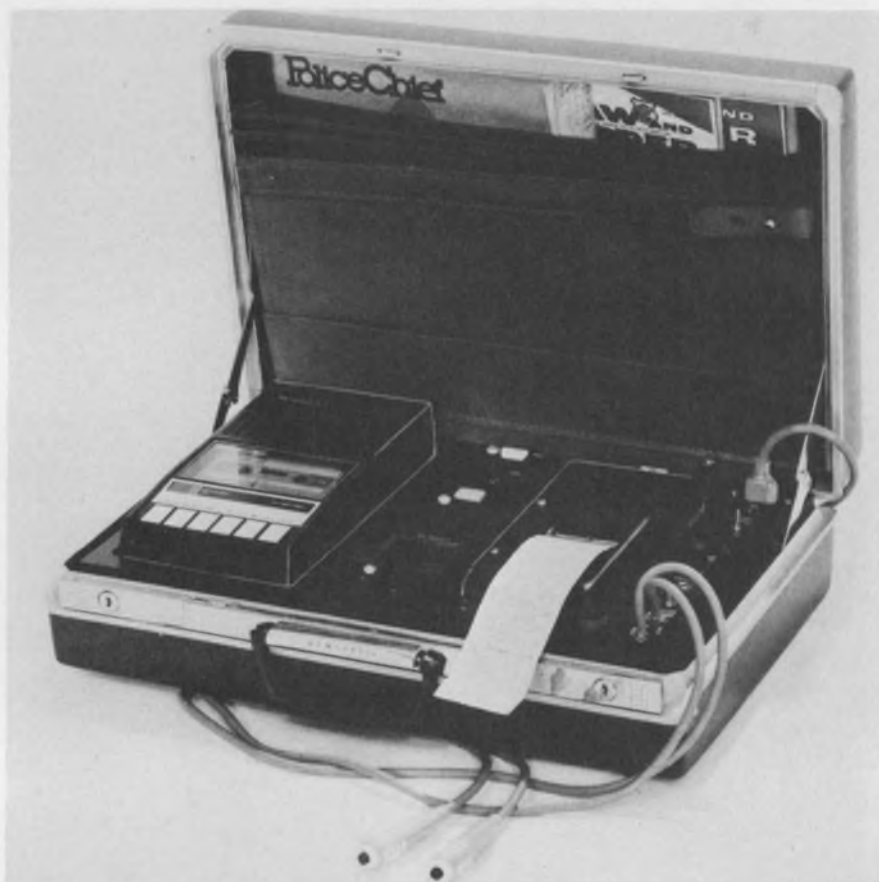
By detecting the emotional stress in a person's voice, the voice analyzer can help determine whether someone is lying.
