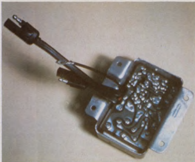
Fillers such as sand can lower costs and improve the thermal and other properties of potting compounds. An automotive electronic ignition system, shown before and
