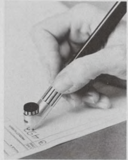
Computerized pen automatically translates hand-printed data into ASCII-coded data. The pen is designed to replace keyboard entry devices now used.
