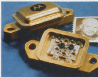
A wide-band, low-noise cable television amplifier, the Motorola MHW 526, produces 16 dB of gain from 40 to 300 MHz. Input and output impedance is 75 Ω.
