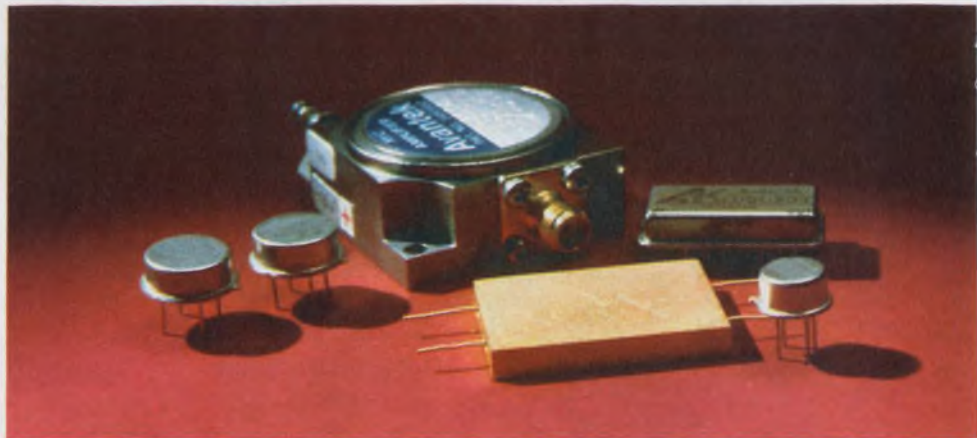
The wide variety of packages used for MICs is shown in this array of products from AvanteK. They include a 5 to 500 MHz amplifier and a varactor-tuned oscillator each in a TO-5 can. Amplifiers operating from 100 kHz through 4 GHz are also shown in various forms.
