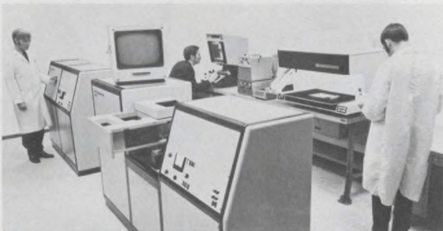
Optical computing is used in this automated fingerprint-identification system from McDonnell Douglas Electronics Co.
