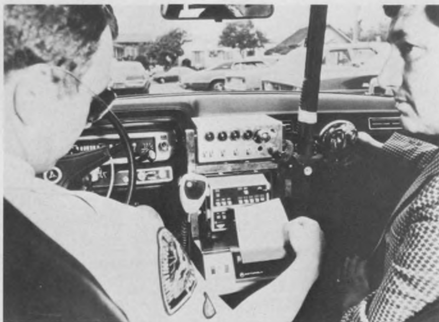
Hard-copy readout is provided as part of Motorola's Command and Control digital-communications system. It minimizes the chance of error in the dispatching of officers to a particular location.
