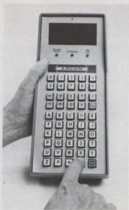
The smallest mobile terminal available is the MCT-16 from Atlantic Research. The unit features a full alphanumeric keyboard plus 10 special-function keys.
