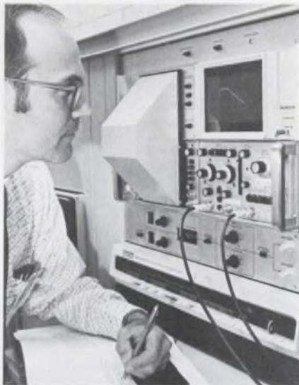
The Sandia vidicon digitizer is checked by Thomas Evans, one of the developers. At top is the display, and below it the digitizer and computer.
