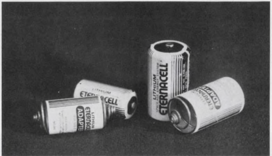
Lithium batteries from Power Conversion have a shelf life in excess of five years. Because of the 3-V cell, one battery can replace two carbon-zinc units. A spring-like adapter takes up the extra space.
