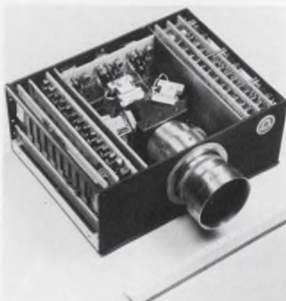
A prototype color TV camera that uses three 220-by-128-element, charge-coupled-device arrays has been built by Bell Laboratories.
