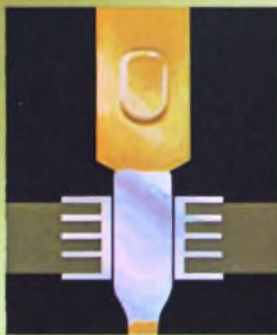
Solder band is pulled into through-hole with just enough force to retain it during reflow.
