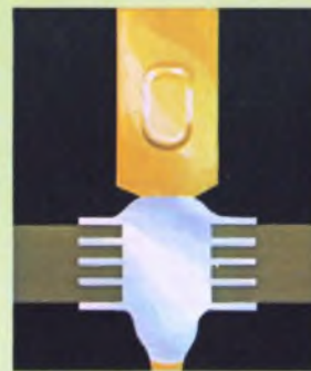
Contact is flow soldered in place, producing uniform fillet with full solder, top to bottom, and clean, solder-free posts.
