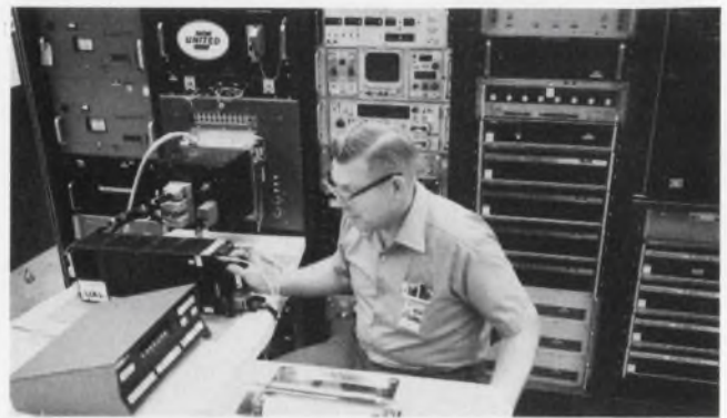
Automatic test equipment (ATE) station at the San Francisco International Airport checks out a digital air data computer in a United Air Lines DC-10. Session 13.
