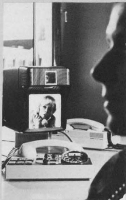
Videotelephone unit has a 28 sq-in. screen and a vertical resolution of 267 lines.
