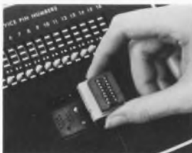
insert different device socket if necessary.
