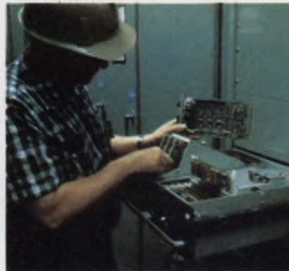
Printed-circuit board triggers an alarm when a seismic device settles on its newly installed base.
