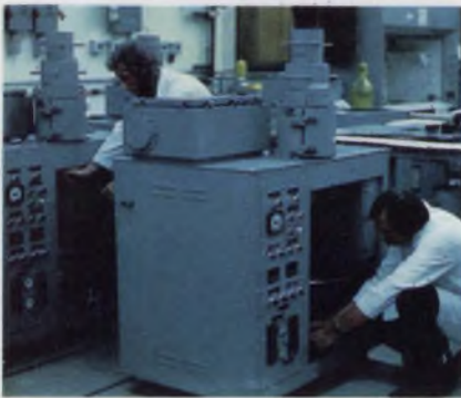
Remote radiation monitors contain sodium-iodide crystals and photomultiplier tubes. Gulf Electronic Systems, San Diego, builds them.
