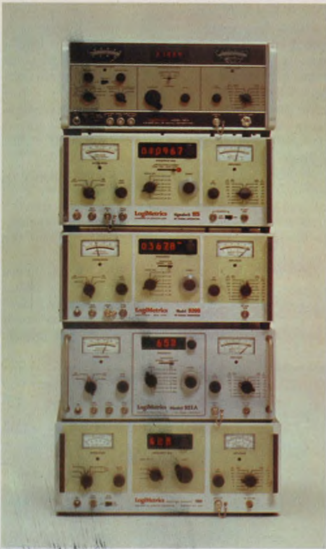
LogMetric's sig gen line ranges from the 750A, a 520-MHz unit with five-digit readout, to the 921A, an 80-MHz unit with a three-digit display.
