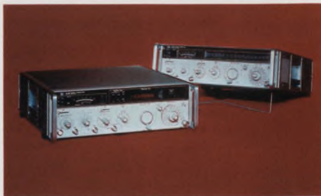
Hewlett-Packard's latest sig gen is the 8640B, a 512-MHz unit with digital locking and internal six-digit counter. Stability in the locked mode is 0.05 ppm/hr.
