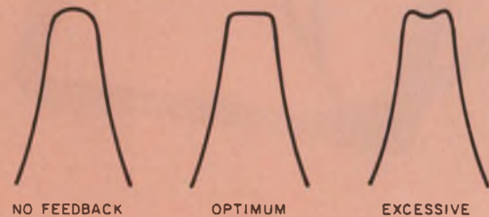
2. Typical filter output response with various amounts of feedback. The range of magnitudes plotted represents 40 dB, and the fractional 3-dB bandwidth is about 2.5%.
