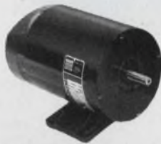
42A Permanent Magnet Motor Line: Standard TENV ratings are \frac{1}{8} , \frac{1}{6} , and \frac{1}{4} Hp at 2500 Rpm. Only 4.3" in diameter. Available with NEMA Type C face mounting shields.
