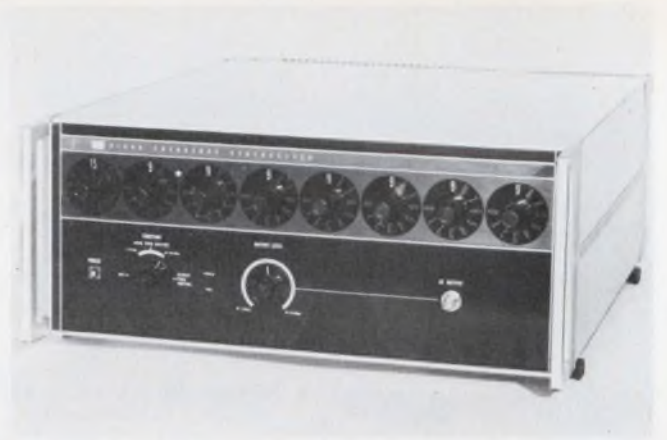
The popular Fluke 6160A indirect synthesizer offers output to 160 MHz, BCD programming with 0.5-ms switching time, and a signal-to-phase-noise ratio of 62 dB.
