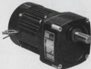
42R-E Induction Parallel Shaft Gearmotor Line: Torques thru 350 Lb-in. Ratios thru 300:1. Helical steel gearing. High overhung and thrust load capabilities.
