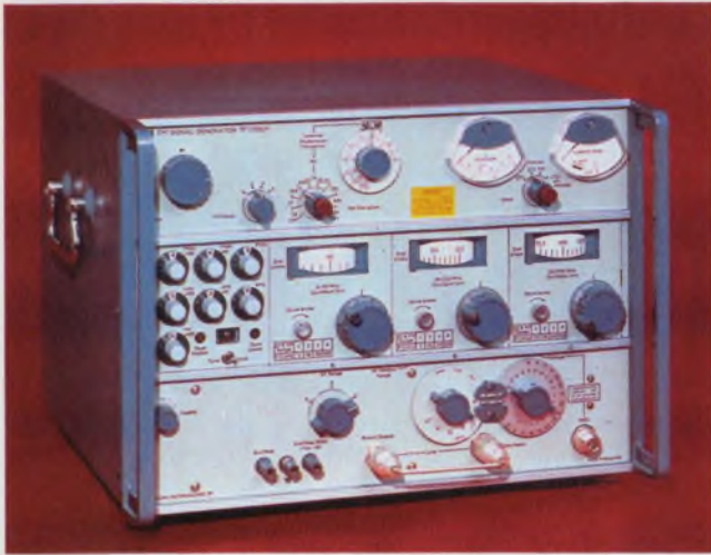
The 2006 uses Marconi's digital synchronizer to lock output frequency over the 10 to 500-MHz range.
