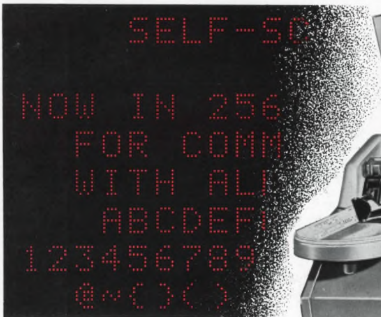
SELF-SCAN Panel Display Subsystem, 256 Character Capacity, 5 x 7 Dot Matrix, Characters 0.25" High. 64-character format, available with all drive electronics including memory, character generator, and timing.
