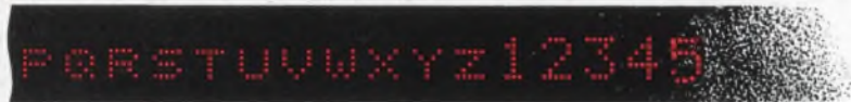
32 37. 80 Character Position Panel, 5 x 7 Dot Matrix, Characters 0.2" High. Alphanumeric panel with 64-character format.
