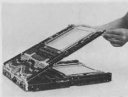
Wire memory from Oki Electric Industry Co. has a capacity of 8192 words, a 200-ns access time and consumes 40 W.
