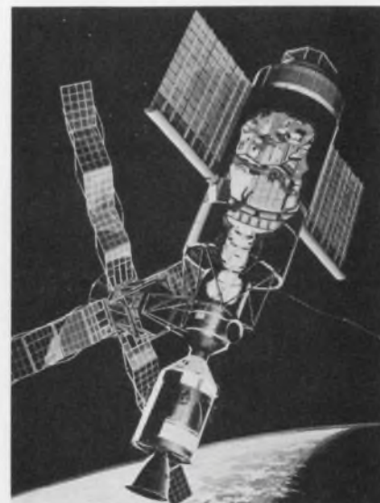
Skylab, NASA's first manned orbital space station, will be powered by two giant solar-cell arrays.
