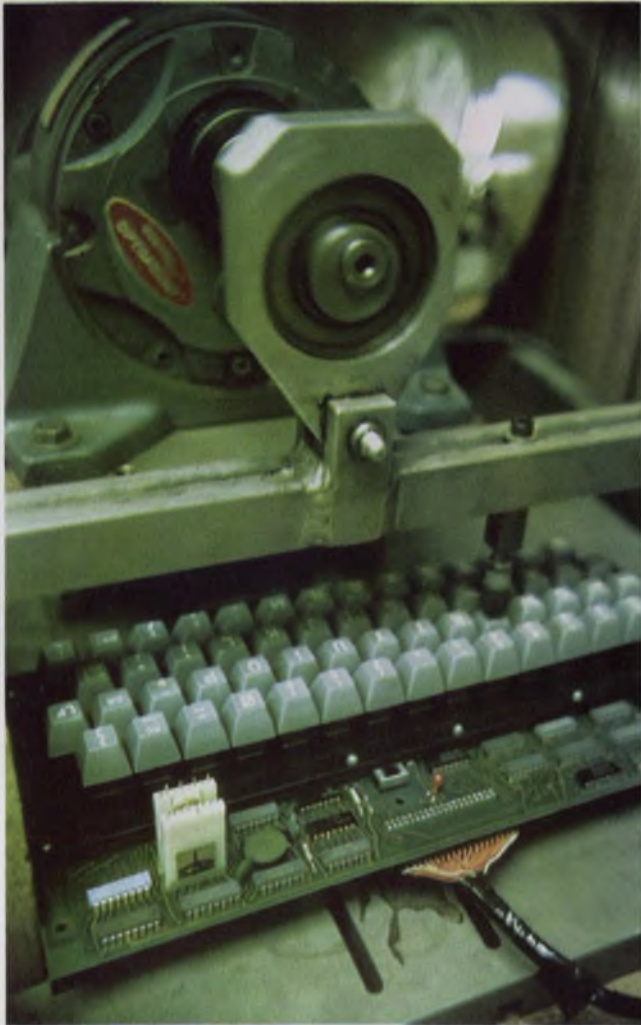
Donnelly Mirrors evaluates the lifetimes of its flexible-diaphragm keyswitch on this test rig.
