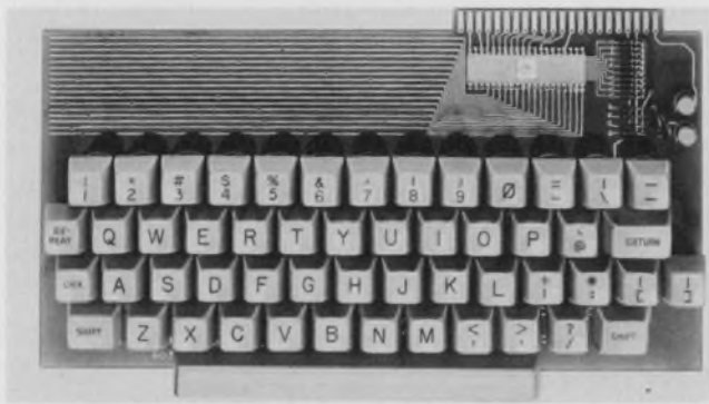
MOS-encoded keyboard (above) from Maxi-Switch uses a single DIP to provide any eight-bit code. Contrast this
