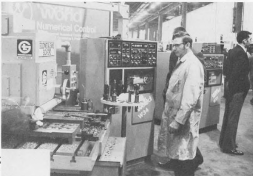
New World C-Line computerized numerical control system, introduced by Westinghouse, is said to provide "first all-stored logic numerical control."
