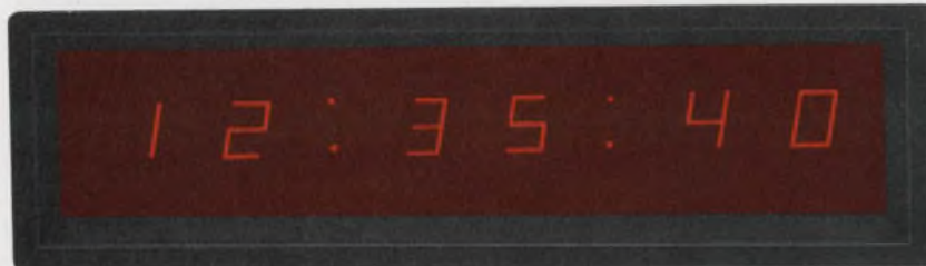
MAN1 — The standard of the industry, the .27" MAN1 is mounted on a 14-pin DIP and encapsulated in clear epoxy. Directly compatible with IC's, it is being used in a wide variety of alphanumeric display sockets. (Shown in a demonstration clock face.)
