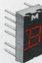
MAN1002 — A .27" 7-segment hexinumeric display, the MAN1002 provides all numbers and the letters A, B, C, D, E, F, H, I, J, L, O, P, S, and U for digital and cockpit readouts that require this capability. Like all our GaAsLITE displays, it is shock resistant and impervious to vibration.
