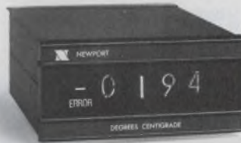
SERIES 260 DIGITAL THERMOCOUPLE INDICATOR: For TC types J,K,T,S,R,E and RTD's 1° resolution • °F or °C • -310° to +3100° F • BIGS-BCD outputs • 2½" H x 5" W x 6½" D.
