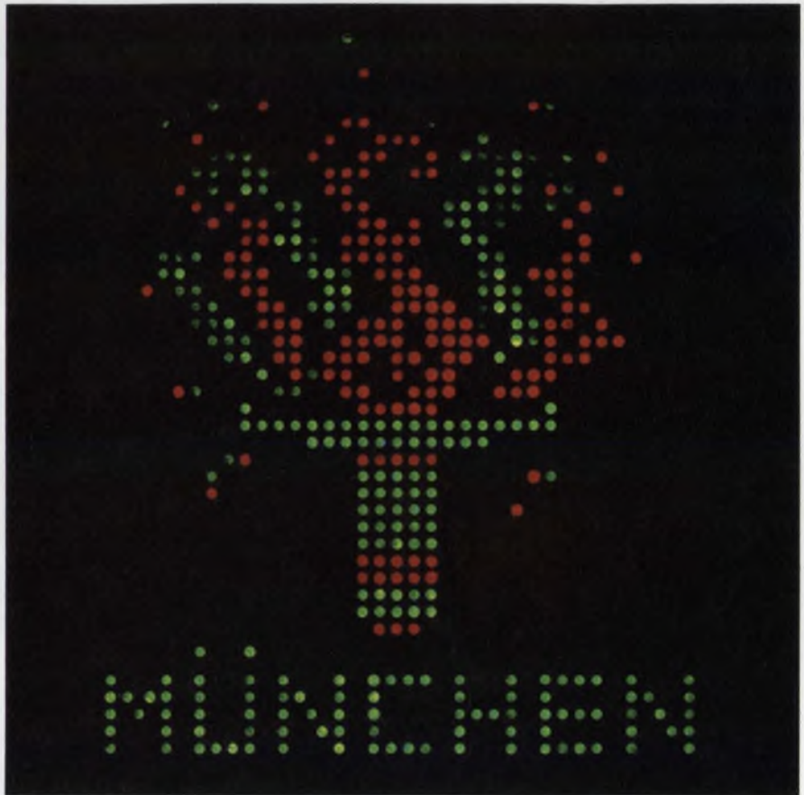
An animated display of the Olympic sports torch consists of electronically controlled arrays of red LEDs and green LEDs of the infrared phosphor-activated type. Matsushita Electric of Japan built the system.
