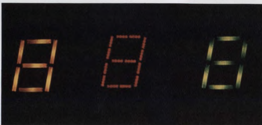
New colored LED displays by Monsanto in a gallium arsenide phosphide yellow (MAN 8) at left, and in a gallium phosphide green (MAN 5) at right, are compared above with the red display industry standard (MAN 1), center.
