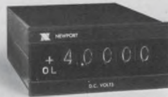
SERIES 2000A DPM: \pm 39,999 counts • DC volts, current or ratio • 01% accuracy BIGS-BCD outputs... buffered, isolated, gated and stored • 2½"H x 5"W x 7½"D.
