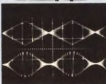
AM—Top: Triangle modulating signal. Bottom: Sine wave modulating signal.
