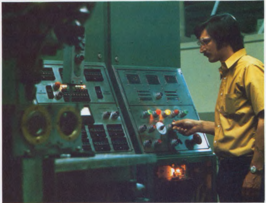
A numerical control system runs a Burgmaster for the precision drilling needed for the casing for the AN/ARA-63 all-weather landing system receiver that Cutler-Hammer's AIL Div. is building for the Navy.
