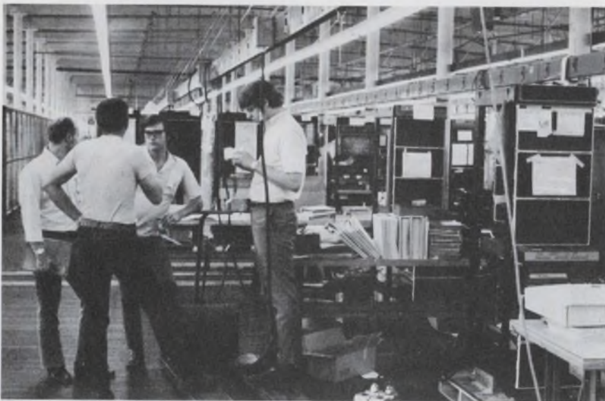
PDP-11/45 computers are being tested before shipment by two PDP-11/20 minicomputers at Digital Equipment Corp.'s plant in Maynard, Mass.
