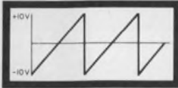
Sawtooth waveform ERMS = 5.77 Volts; 17.4 dBm
