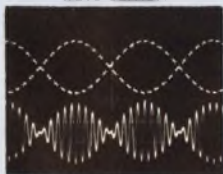
Suppressed carrier— Top: Square wave carrier. Bottom: Sine wave carrier.
