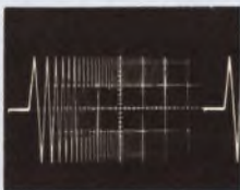
Gated sweep, one burst of swept waveform.
