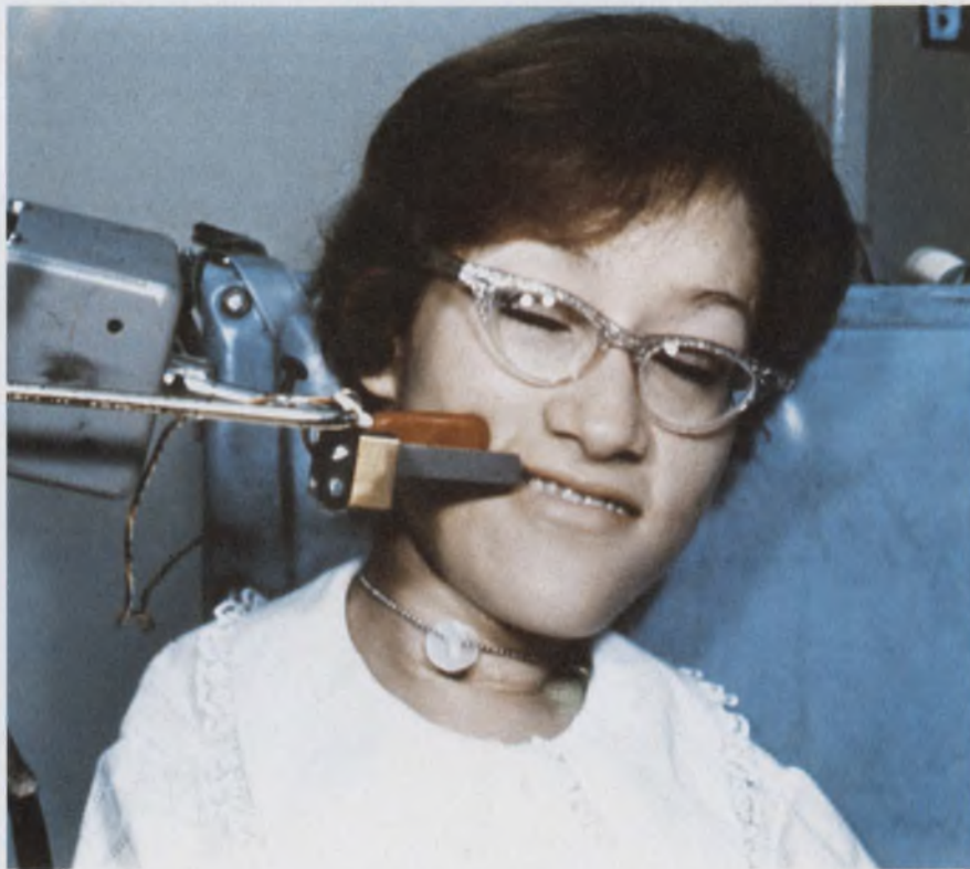
Patient's tongue controls an electric wheelchair by operating a proportional-control system that has strain gauges mounted on cantilever beams.
