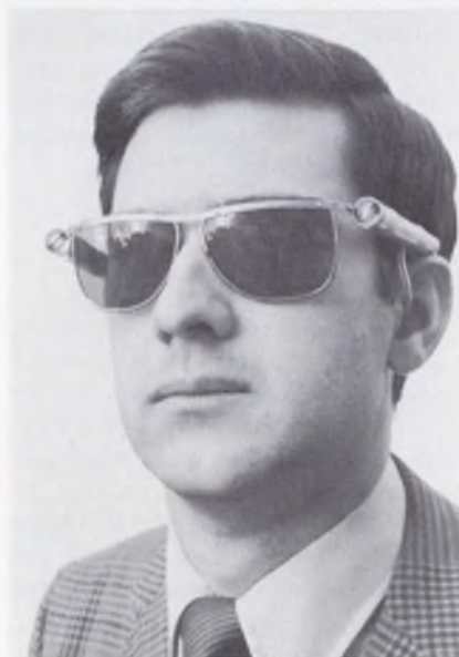
Optical radar system to guide the blind can be mounted on glasses.
