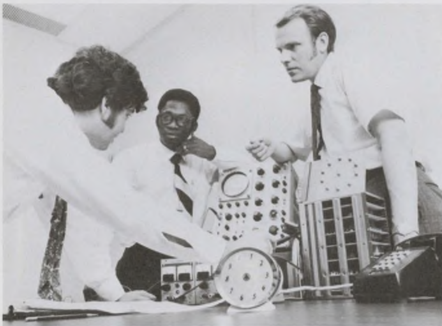
A voice-controlled telephone dialer being developed by Bell Telephone may someday allow handicapped people to dial by speaking into a microphone.
