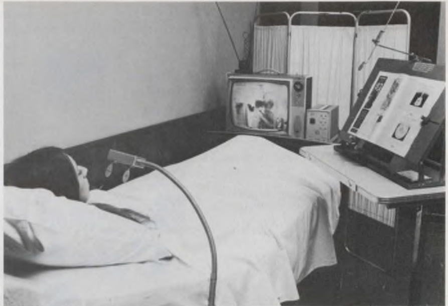
A breath-operated switch and control system developed by NASA enables paralyzed patients to operate appliances by simply blowing on a switch.
