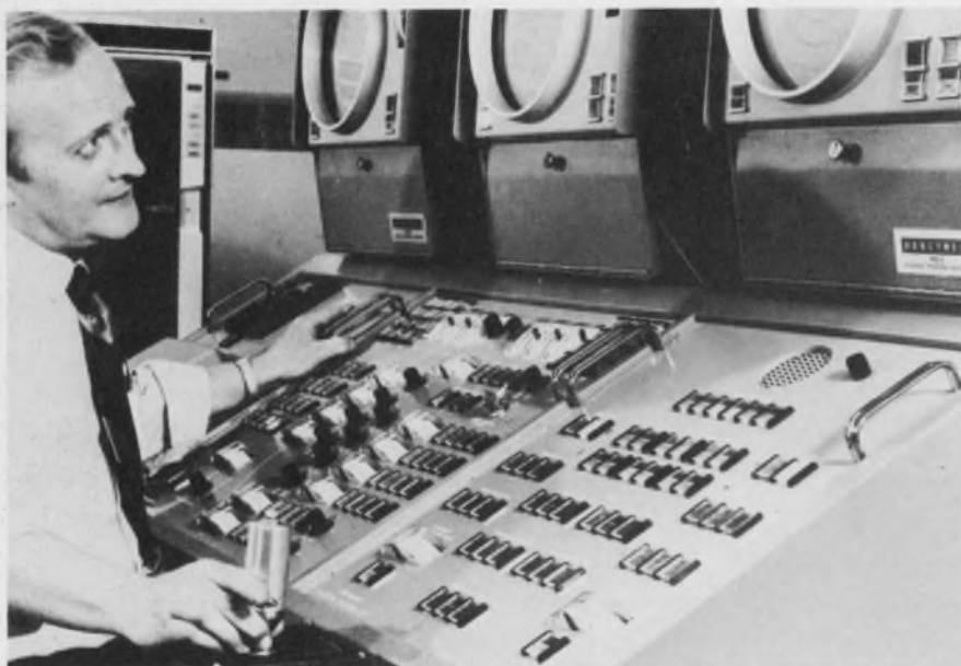
Automatic station-keeping of the ship will be controlled at this Honeywell H-316 console with position-location displays for monitoring.
