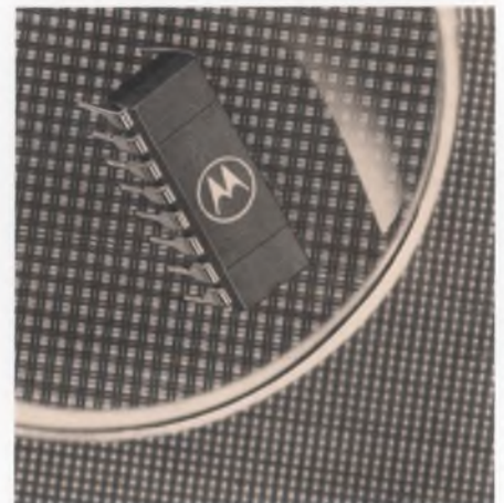
Fast, high-gain sense amp — MC1544 — has level-restoring circuit to maintain TTL levels on its output at the highest repetition rate.
