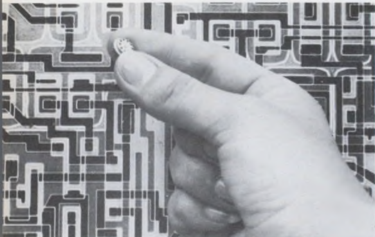
The first monolithic phase-locked loop, part of the Signetics 560 series, lends itself to a wide variety of applications that formerly required inductors.
