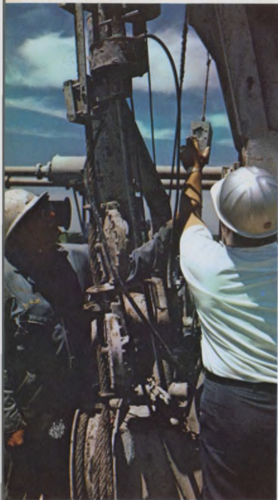
The rig driller watches a Baroid logging supervisor install and calibrate a hook-load transmitter transducer—a potentiometer similar to those used to measure pressure. Accuracy is \pm 500 pounds/250,000 pounds.
