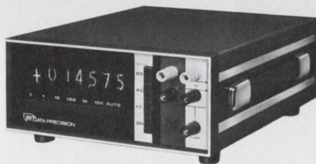
Model 2540, 5½ digits. DC volts, AC volts, Resistance, Voltage Ratio. Auto-ranging. Auto-Polarity. Isolated BCD outputs. Remote triggering. Remote ranging. Basic accuracy \pm 0.001\% f.s. \pm 0.007\% rdg \pm 1 l.s.d. for 6 months. One-piece price: $1,195.00
