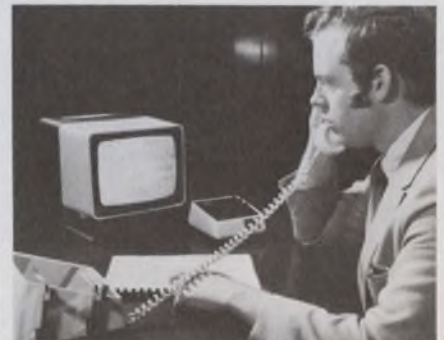
Video-Voice system developed by RCA will transmit still pictures over voice channels.
