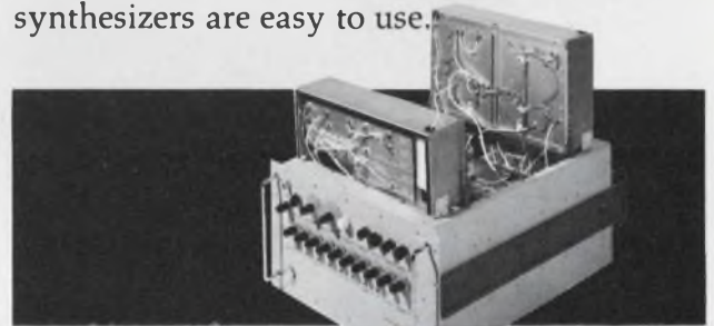
Model 645M with swing-out trays opened to demonstrate access to modular circuitry.
