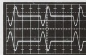
Single shot—sine wave output using pulse mode, start-stop control at 0°. For phase relationship studies.
