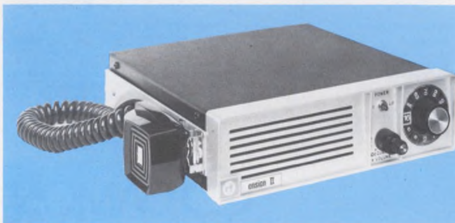
Ensign II , vhf-FM radio-telephone built by RF Communications, Inc., can operate with a coat hanger if the antenna is lost.
