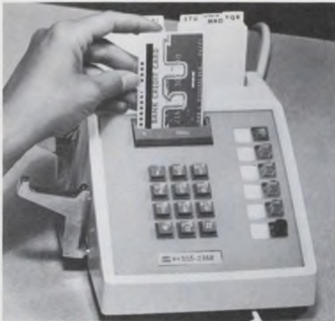
New standard-size credit card designed by Bell Labs engineers for credit verification via telephone.
