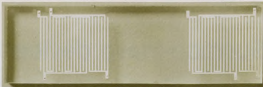
This filter can be used to encode or decode a digital signal. It was developed at MIT Lincoln Laboratory, Lexington, Mass.
