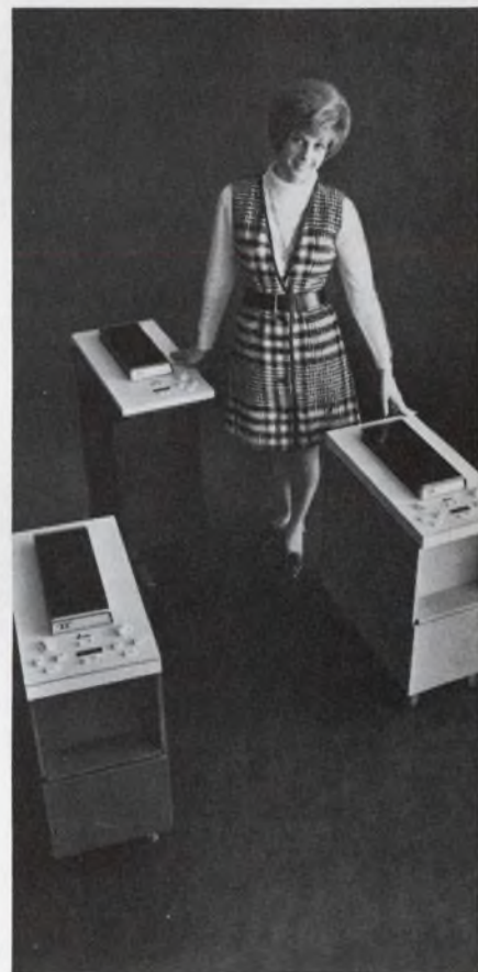
magnetic tape data terminals: Use compact reusable tape cartridges. Operate on-line at up to 2400 wpm, and connect "locally" to lower speed Teletype terminals using ASCII code.
