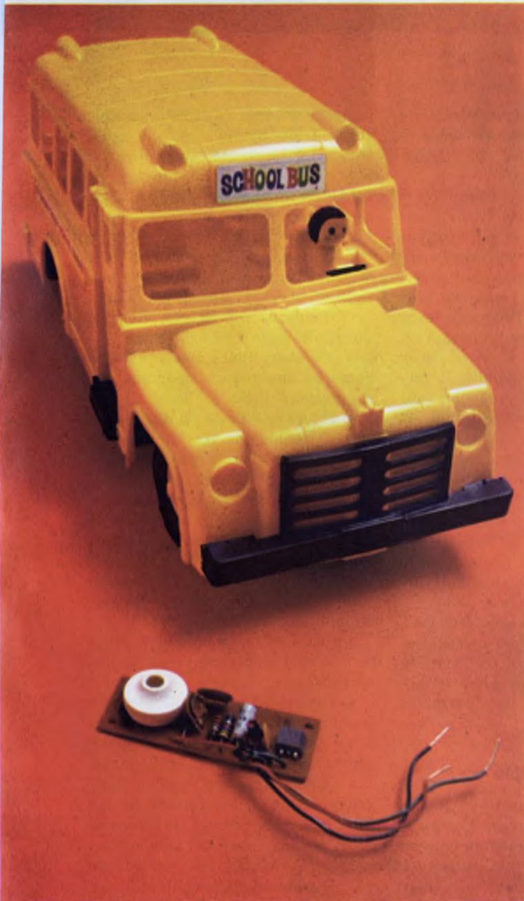
3. At the blast of a whistle, Remco's Tricky Busy School Bus closes its door and starts up. The PC board and circuit shown have an SCR that is triggered by the whistle-signal output of the microphone, amplified by transistor Q1. With the bus stopped, the cam switch is open, and starting motor current flows through the SCR. As the bus moves, the cam switch closes, shorting out the SCR and returning it to a nonconducting state. When the bus stops, the voltage across C1 holds Q1 off for 1.5 to 2.5 seconds.
