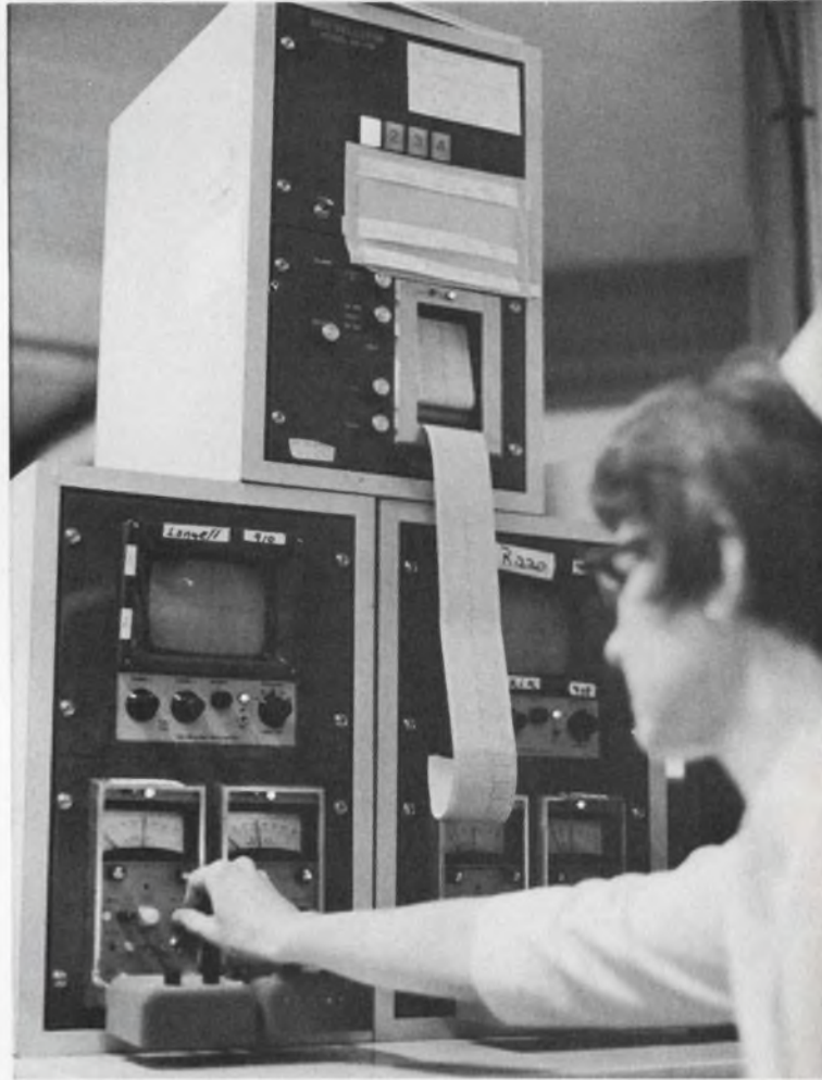
3. This display is located near the telemetry receiver in Overlook Hospital. Oscilloscope and alarm units are mounted below a hard-copy oscillograph which produces a permanent record, like that shown at the top of the page. The use of the scopes and oscillograph is desirable; the alarm units are mandatory.
