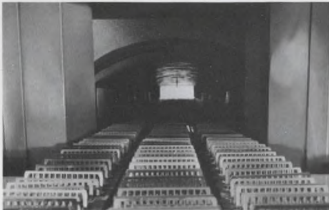
Sealing cerdip at 550° C
