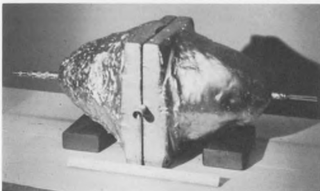
This experimental prolate spheroid resonator is symmetrically excited by the magnetic coupling loop. The
