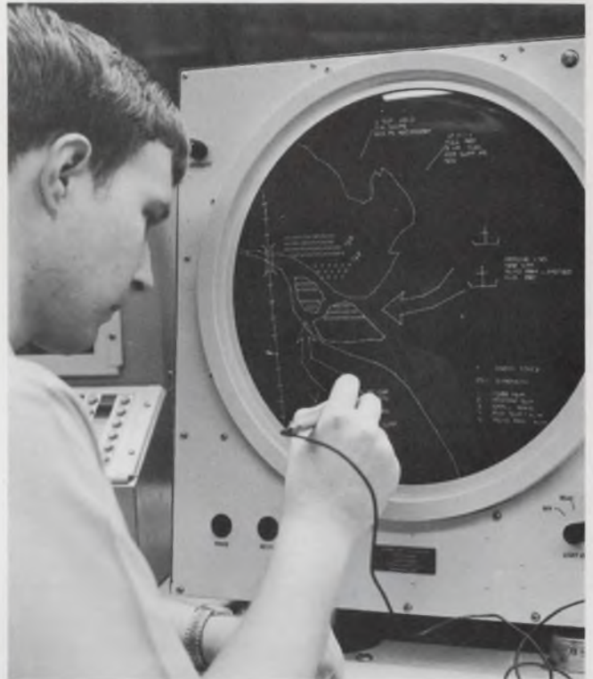
A radar monitor scope with interactive graphic capabilities has properties useful in military or civilian applications. The display is computer generated.
