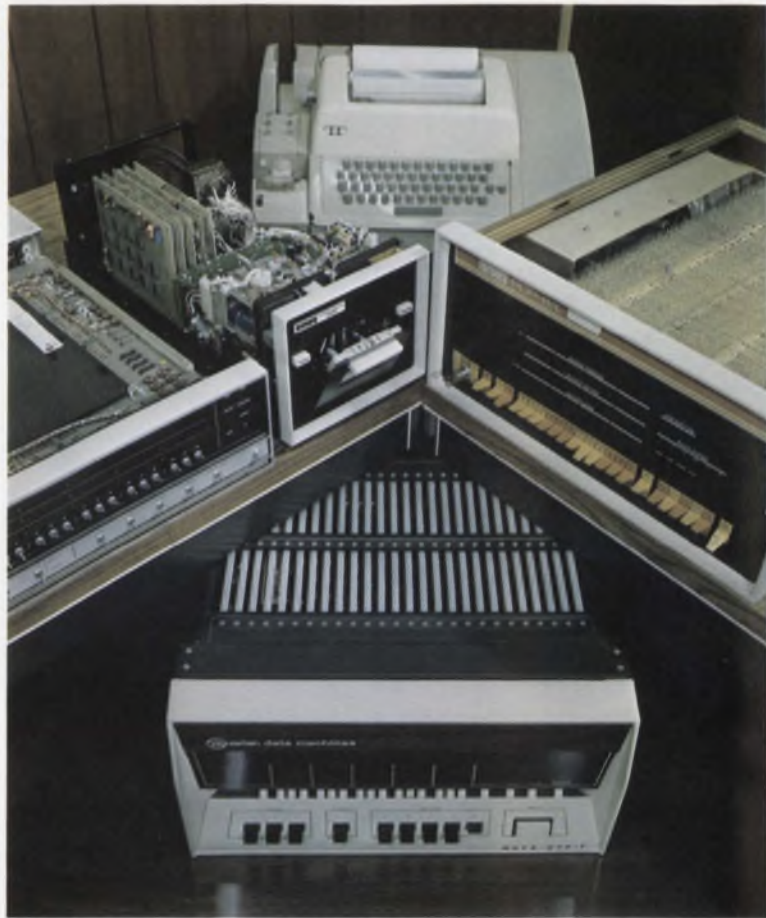
Low cost peripherals designed for use with minicomputers are recent arrivals on the scene. The cassette tape recorder shown accompanying some of the mini-computers it operates with, is one of this new breed.
