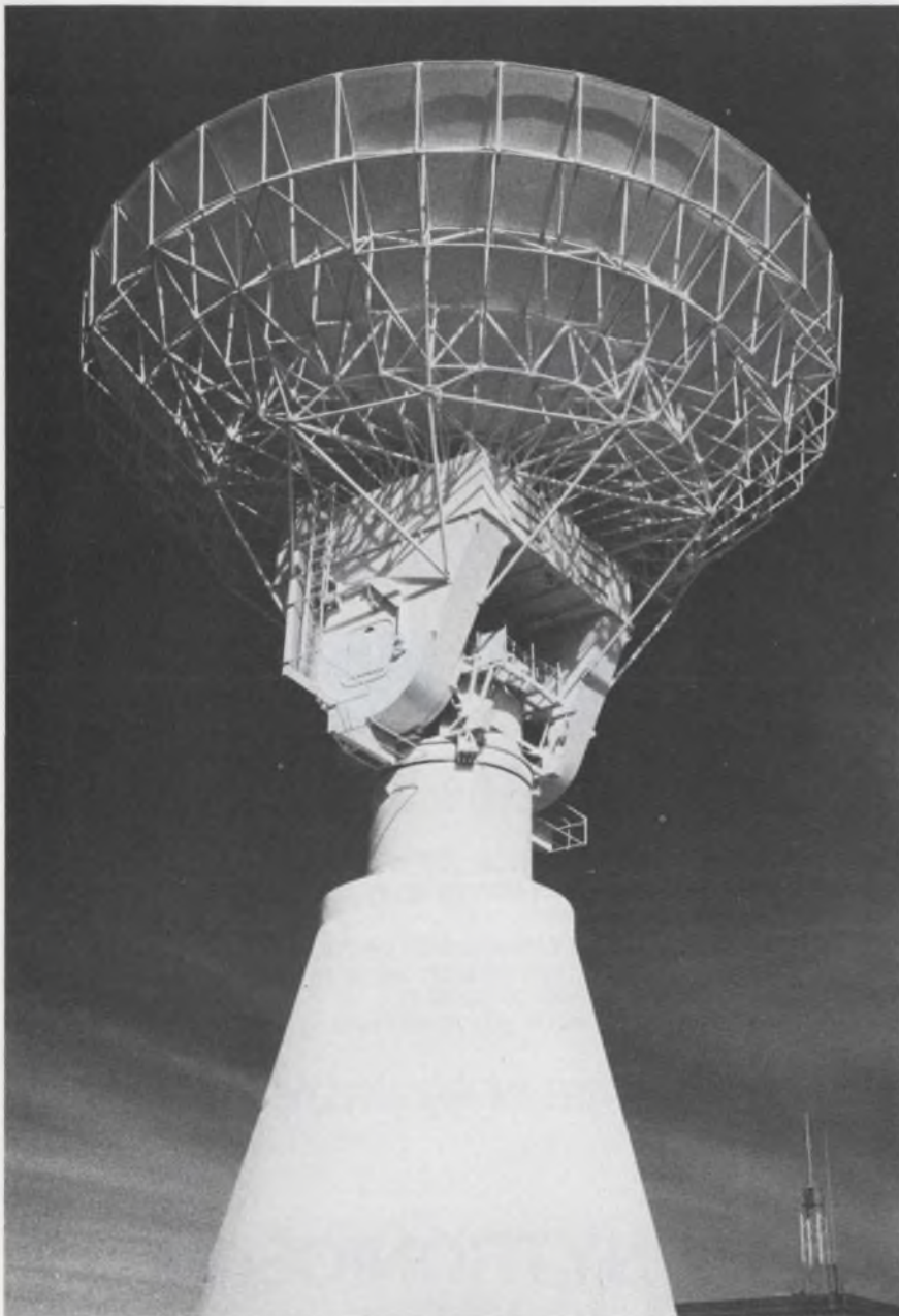
Rampart S-band radar acquires reentering payload, measures cross section and trajectory, then passes directional data on to RAM radar.
