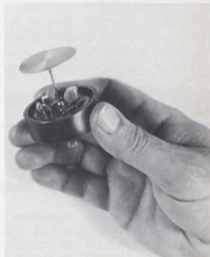
A disc-topped rod plus electronics make up the Voltage Probe Antenna
