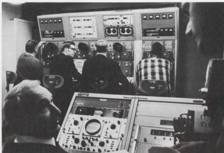
A-scope (foreground) in RAM radar blockhouse shows cross section of a 12-inch sphere released by Loki rocket at 230,000 feet.
