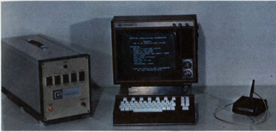
Remote console made by Computer Communications, Inc., shows that the present TV set can be used as a computer terminal.
