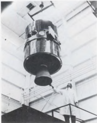
ATSS-V during final tests at Hughes Aircraft Co., El Segundo, Calif. Prior to launching on Aug. 12, 1969. The rectangle with a dozen small circles at the upper right section of the satellite is the antenna portion of an L-band communications and navigation system.
