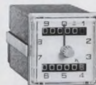
T3B —Double scale use-time indicator—99,999.99 hours total time and reset time. Tenths in red, hundredths with sweep hand. Reset scale knob resettable. 115 V., 60 hz. Panel mount. 1.87" square.
