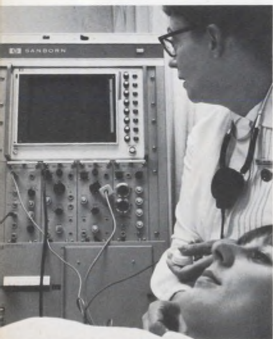
Phonocardiogram , used to obtain a visual image of the sounds of the heart as it pumps, is demonstrated by Lorraine Gillard. The equipment detects murmurs and other heart disorders.
