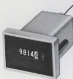
Model T4B —Miniature use-time indicator. Scale to 9999.9 hours, with tenths in red. Non-reset. 110 V., 60 hz. Panel or bracket mount. 1.59" wide.
