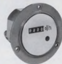
Model T5BB —Economical use-time indicator. Scale to 9999.9 hours, with tenths in red. Non-reset. 110 V., 60 hz. Panel mount. 2.88" dia.
