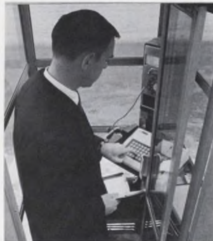
Portable terminal in an attache case will permit users to "talk" to a computer from any standard telephone.
