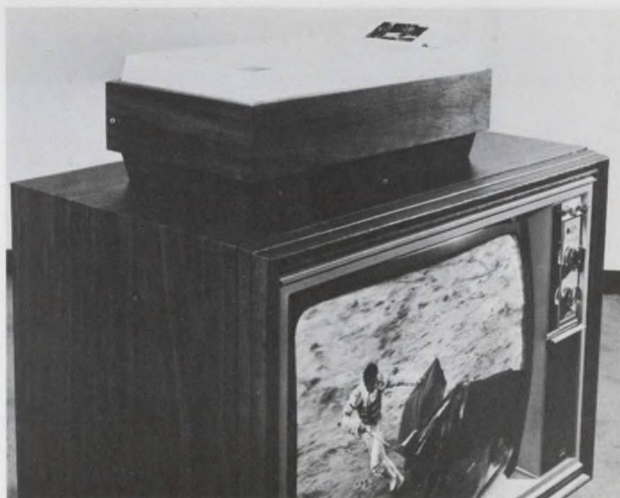
A designer's concept of RCA's SelectaVision TV tape player sits atop a standard color receiver. Cartridges of proposed low-cost color tapes are inserted in the unit at the top right.
