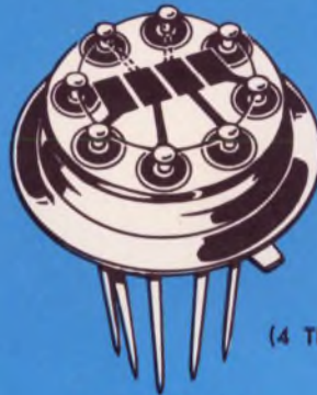
4 POLE 65 MHz TO-5 PACKAGE
