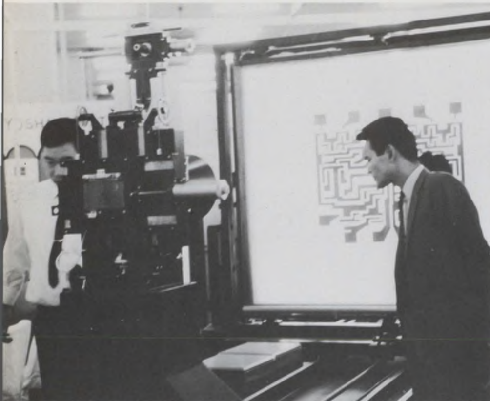
Photo-mask reduction camera was exhibited by Dai Nippon Screen Co. at recent Japan Electronics Show in Osaka.
