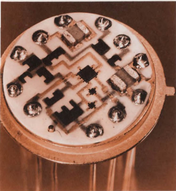
Beam leads offer easy bonding and bond inspection, with a resultant increase in hybrid yields. Photo of a buffer-limiter circuit, employing a beam-leaded op amp and two 1N914 beam-leaded diodes on an aluminum substrate, courtesy Texas Instruments Inc., Dallas, Tex.
