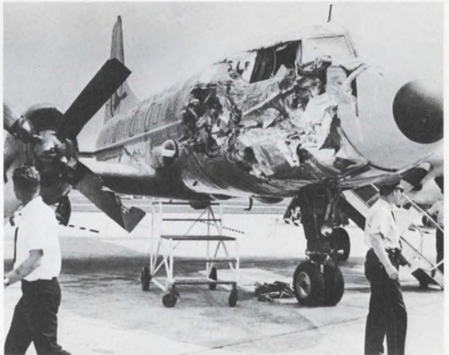
This DC-9 overtook a slow-moving Cessna 150 at Lambert Field, St. Louis, one and a half miles from the runway. Despite radar advisories until shortly before collision, none of the three men in the airliner cockpit saw the light plane.
