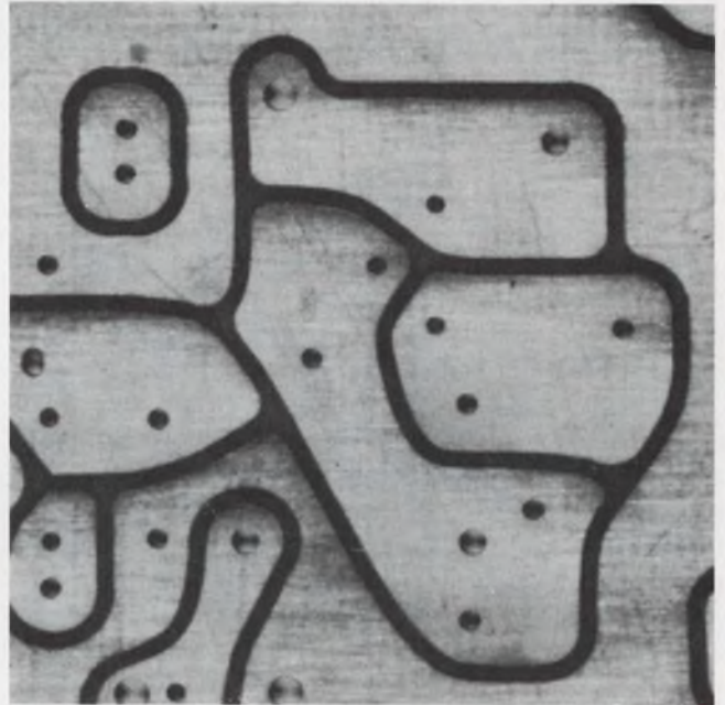
Reduce stray reactances with the boundary method of layout. p. 98.
