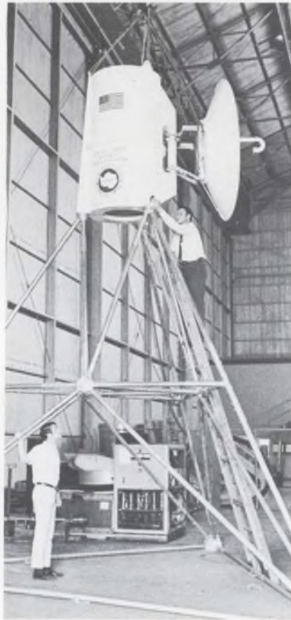
Antarctic observatory capsule and its 15-foot-high pyramidal mount are getting finishing touches.
