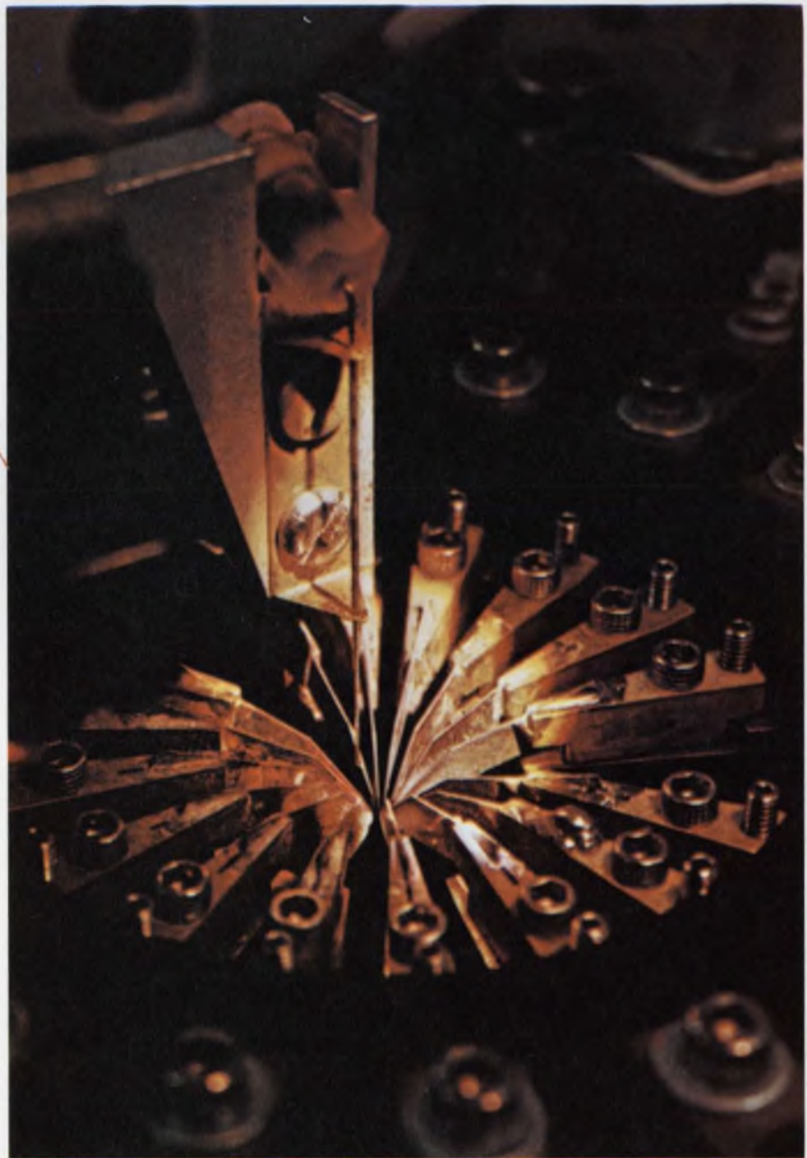
A complex array for dc and functional testing is probe-tested on the production line at Fairchild Camera and Instrument Corp.
