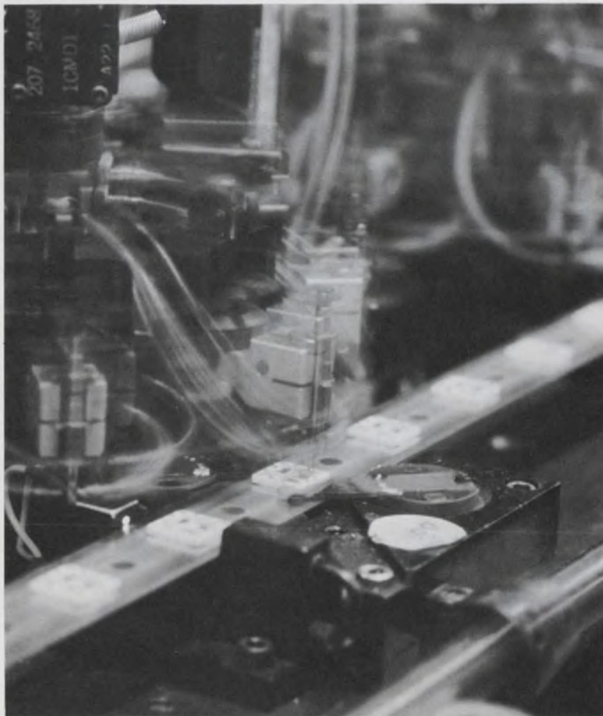
Chip transistors and diodes are placed on alumina substrate at IBM's solid logic manufacturing facility, Hopewell Junction, N.Y. (Paper 2/1).
