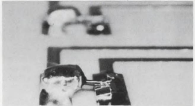
Solid tantalum chip capacitors end high-temperature limitation problems. p. 140.
