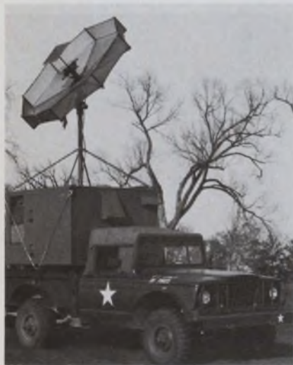
Mobility for the terminal of tactical communication satellites is provided by 1-1/4-ton truck.
