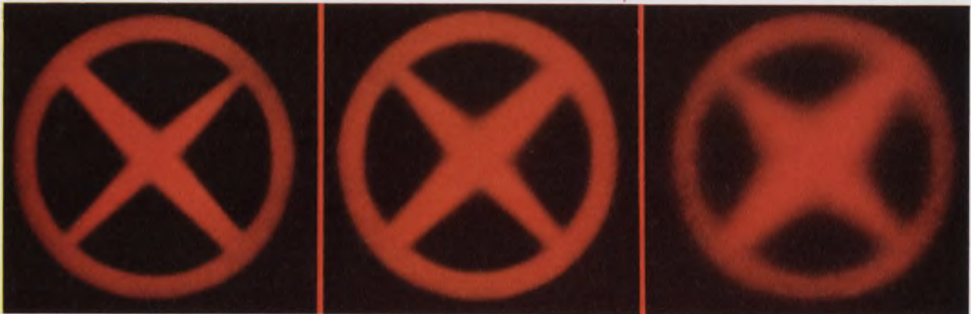
Reducing the redundant information content of a hologram also decreases either the field of view or the resolution (as shown here in successive data reduction
