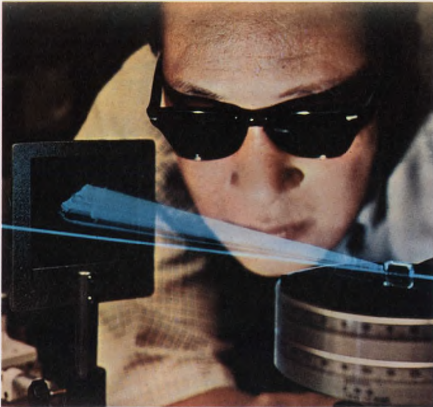
Lithium niobate crystal stores as many as 1000 holograms—but potentially many more—in a lithium niobate crystal. Fong Chen of Bell Laboratories reconstructs one such image. To get a new one, he simply changes the angle at which the laser beam enters the crystal.
