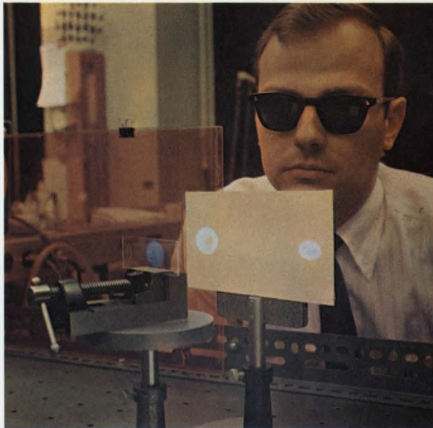
The two bright areas on the card illustrate the high efficiency—over 90%—with which a simple pattern formed in a new holographic material, dichromated gelatin, diffracts a laser beam directed by T. A. Shankoff of Bell Laboratories. The company hopes to store up to 10^8 data bits holographically on a glass slide coated with the emulsion.
