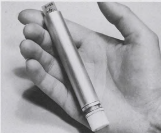
Logic pulse indicator , which goes out to 10 MHz, identifies 50-ns pulse widths, p. 148.
