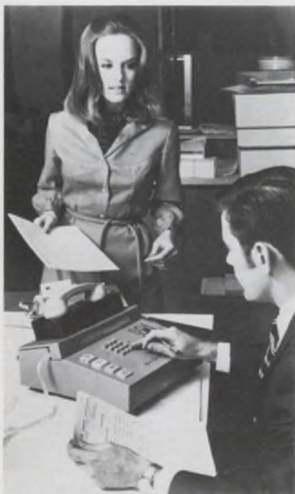
Fully portable computer terminal with hard-copy readout moves data at 10 characters per second.
