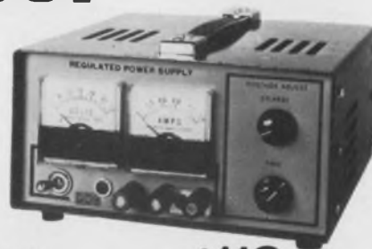
BP-118 0-34 volts at 1.5 amps for
