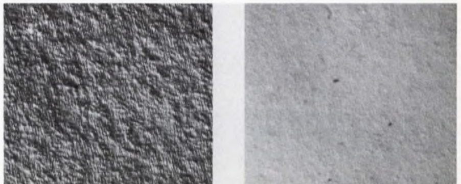
Chemically etching the emulsion gives a smoother surface (right) than conventionally processed hologram, as seen under 250X magnification. This technique is claimed by IBM to give phase-type holograms that diffract 40% of the laser beam into usable reconstructed images. Previous claims of 40% were accompanied by poor S/N.
