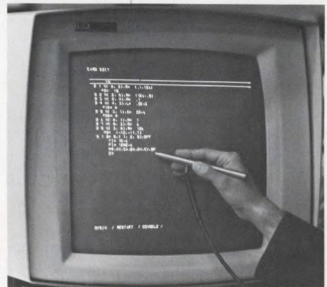
6. The operator may request a card edit to translate the circuit diagram into ECAP source statements.
