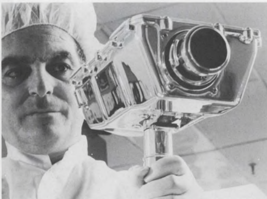
Westinghouse 7-1/4-pound moon camera passed its first flight test in Apollo 9. It uses a SEC tube for adaptability to changing light conditions.
