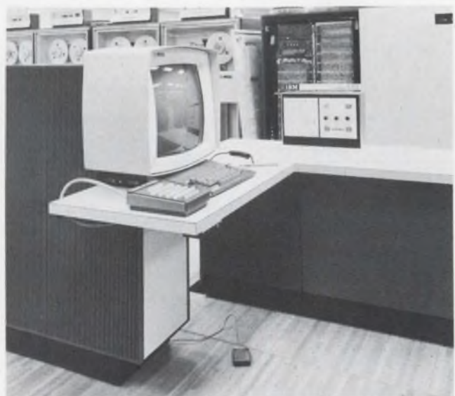
1. The display console of a graphic data processing system includes an operator display unit, a light pen and a keyboard.
