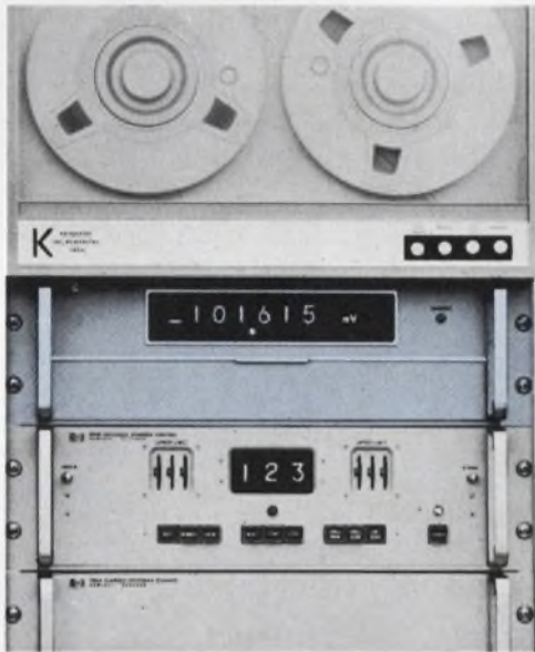
Cover protects 2402A controls for systems use.
