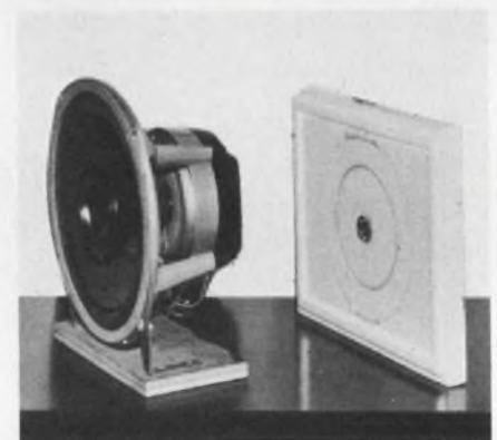
Wafer speaker is a fifth the depth of a cone type, yet handles same power.
