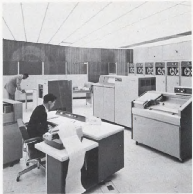
5. The manager of the ILLIAC IV will be a B6500 computer. Its functions will include executive control, I/O processing, peripheral-equipment control, fault recovery, and program assembly and compilation.
