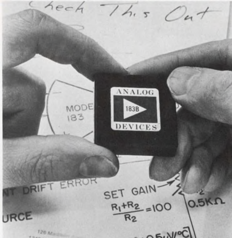
Diff-amp drifts less. A dual-transistor input circuit keeps its stability down in the picoamps. Page 128
