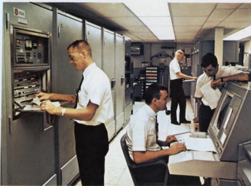
Saturn V checkout is done by these RCA 110A computers at Cape Kennedy. About 4500 different measurements are monitored by similar computers in the Apollo program.
