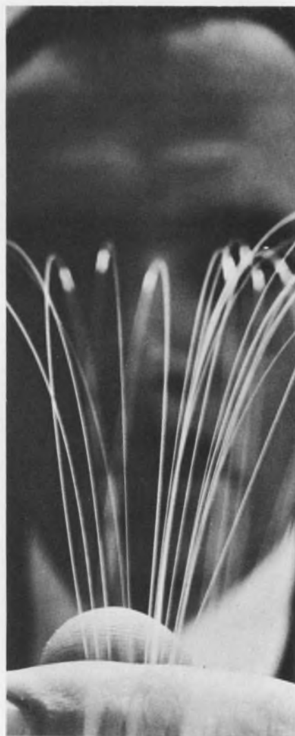
Nonmetallic fiber has a modulus of elasticity of 70 million lb/in. 2
