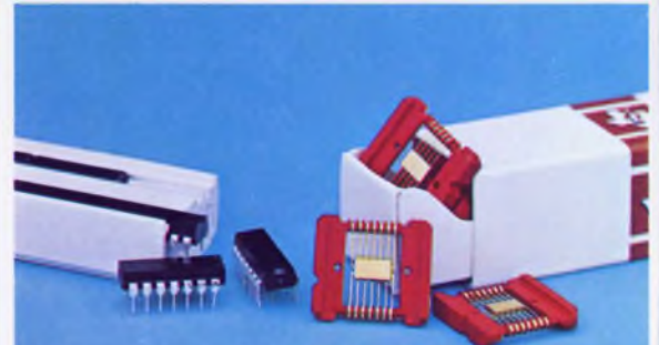
Series 54H/74H offered in both dual-in-line and flat packages
