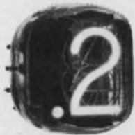
CK1904—Interchangeable with B59956 and NL809.
