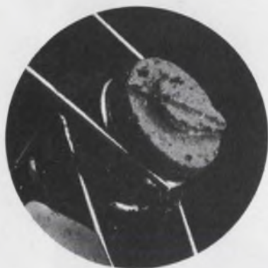
Brush assembly of conventional synchro after 1000 hours
