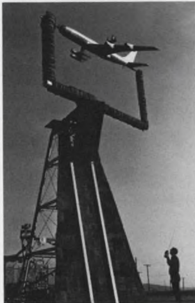
Model of Boeing Co.'s jet transport, designed to carry Air Force's proposed airborne warning and control system, is tested for quality of antenna reception.
