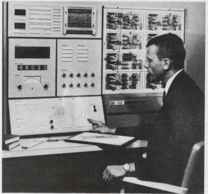
Desk-top analog computer expandable to full hybrid using an external digital computer. Page 101
