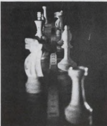
Chess pieces spaced 6 inches apart are encompassed in one hologram.
