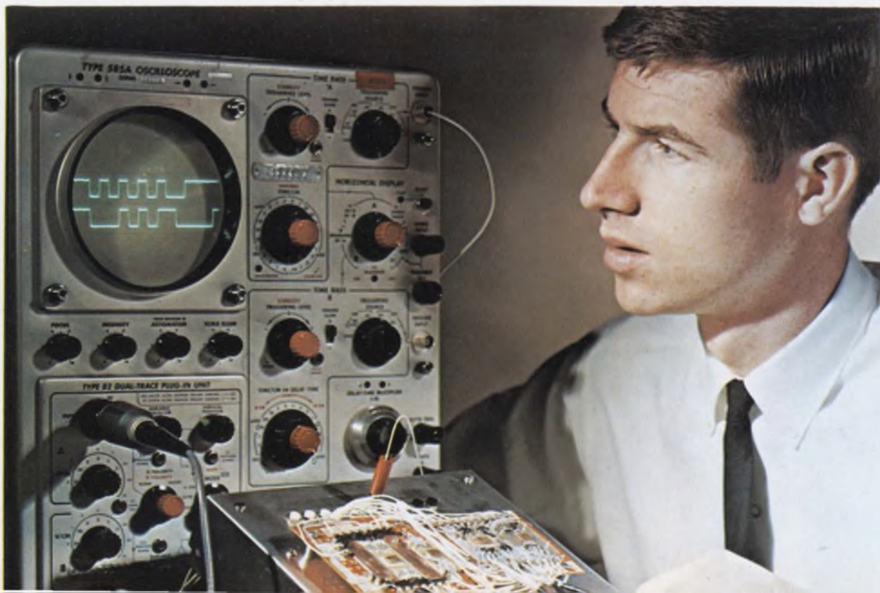
Testing the digital sine-cosine generator, Jim Garvey inspects the two signals on the 'scope that represent the sine and the cosine functions.
