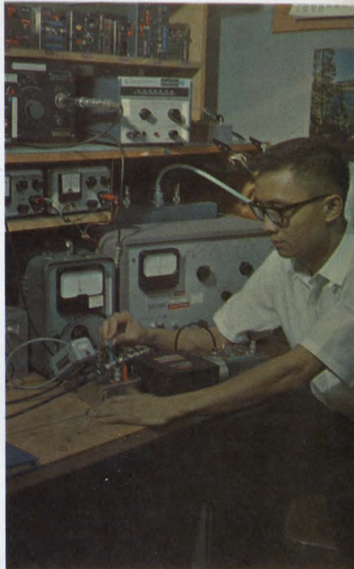
Noise figure measurements on an rf FET mixer are made by Siang Pink Kwok of Motorola Semiconductor, Inc. (Paper 8/1).
