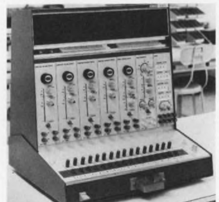
Redcor's model uses a combination of pushbuttons and digital dial settings. Teradyne's ACT I gives an accept/reject decision; Redcor's unit, a direct readout.
