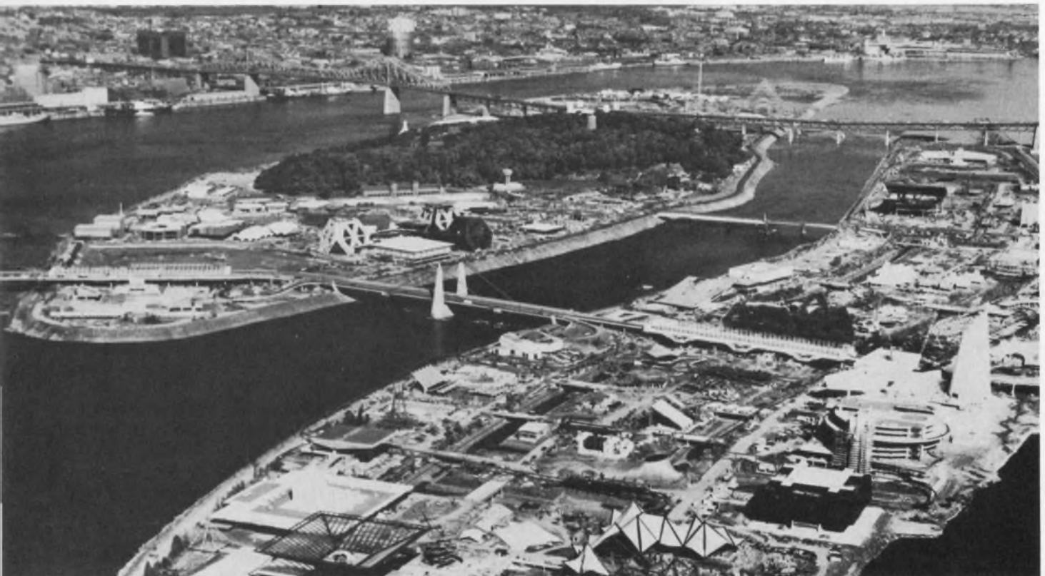
St. Lawrence River serves as site of EXPO 67. Much of the land for the site was artificially created in the river itself. More than 25 million tons of landfill was used to extend an
