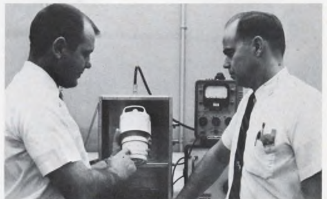
Inserting a power triode into its test fixture, authors Sutherland (right) and Barkley set out to measure the self-neutralizing frequency.
