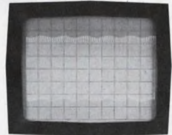
Measure 10 mV, 5 Hz amplitude modulating 1 V, 400 Hz.
