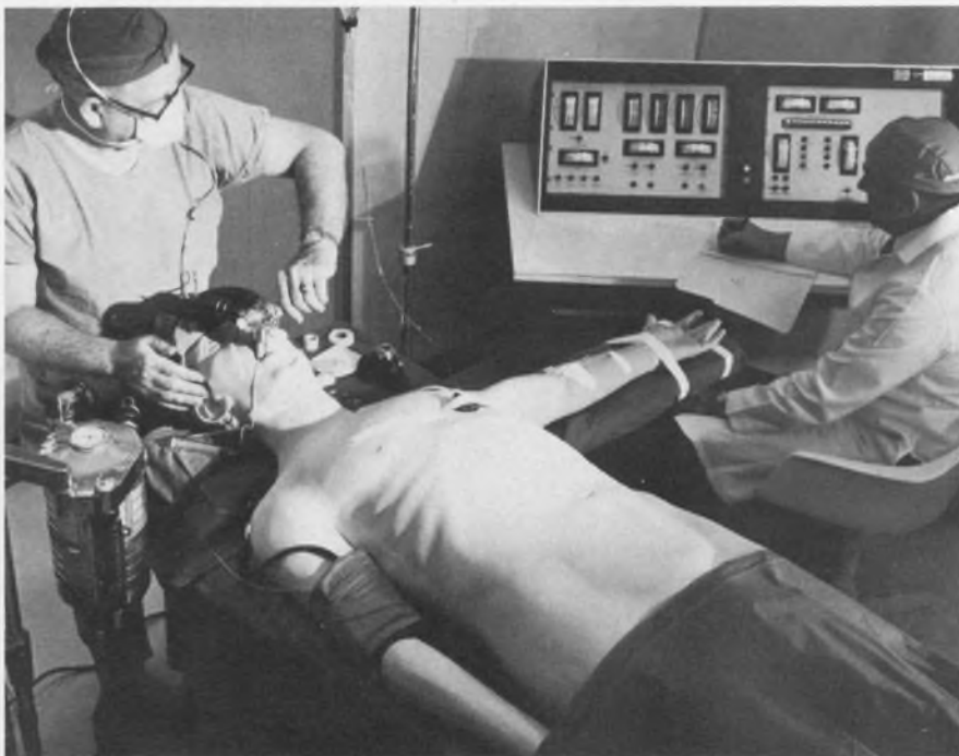
Electronically controlled manikin exhibits all the physical properties of a real patient. Student anesthesiologist is adjusting the oxygen flow while the instructor monitors the procedure from the control console.
