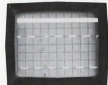
Measure frequency of signal in noise up to 560 kHz by using square wave output, i.e. as a counter preamplifier.
