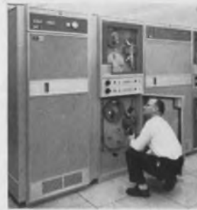
High Speed Data Communications Terminal—unique system extends computer processing facilities to remote locations via broadband transmission.
