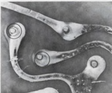
4. Insufficient "wicking" of the solder from the bottom to the top of the wiring board or fracture of the joint due to movement of the lead before solidification are perpetual sources of intermittency.
