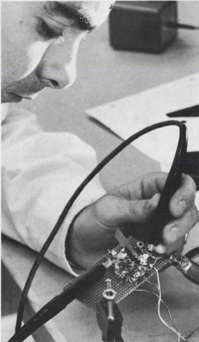
FET scope probe measures response of high-frequency (30 MHz) amplifiers with no loss of circuit's gain.
