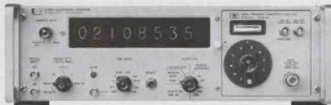
HP Model 5245L Electronic Counter and the 3 to 12.4 GHz Plug-in Frequency Converter
