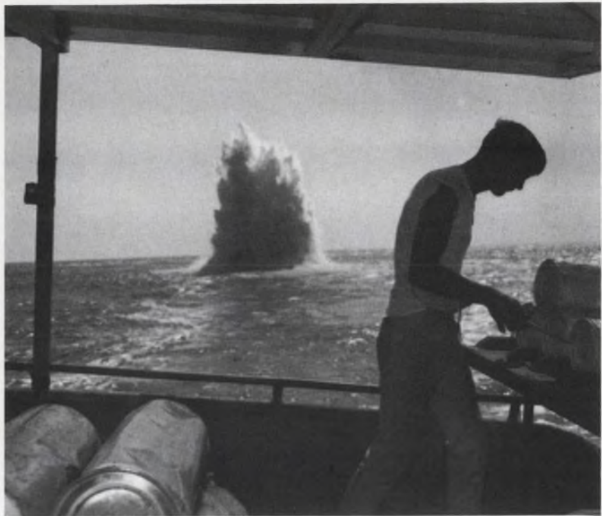
Seismic survey crew from Litton Industries' Western Geophysical Division is shown setting off a marine seismic blast (Science Film Theater)
