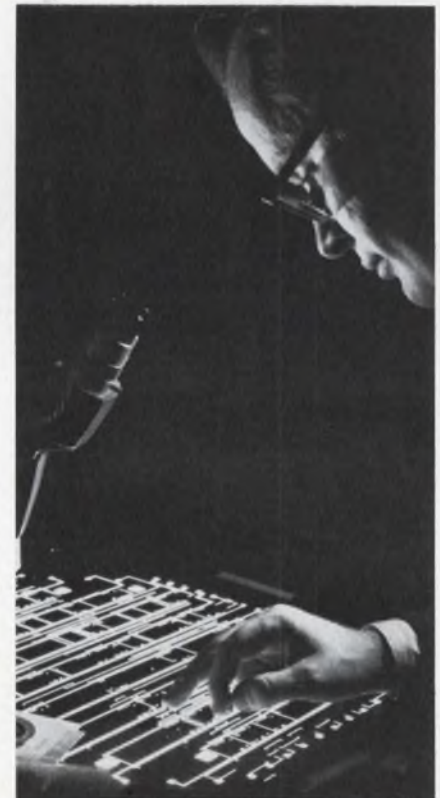
Technician examines enlarged computer-produced interconnection pattern for an array of circuits. The actual array is shown in the foreground (paper 10/2).
