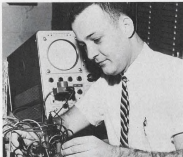
Don't get your wires crossed. Author Hey hooks up his SCR motor speed control unit for a test run.
